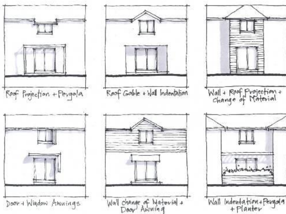
Figure 4 Examples of articulated façade
