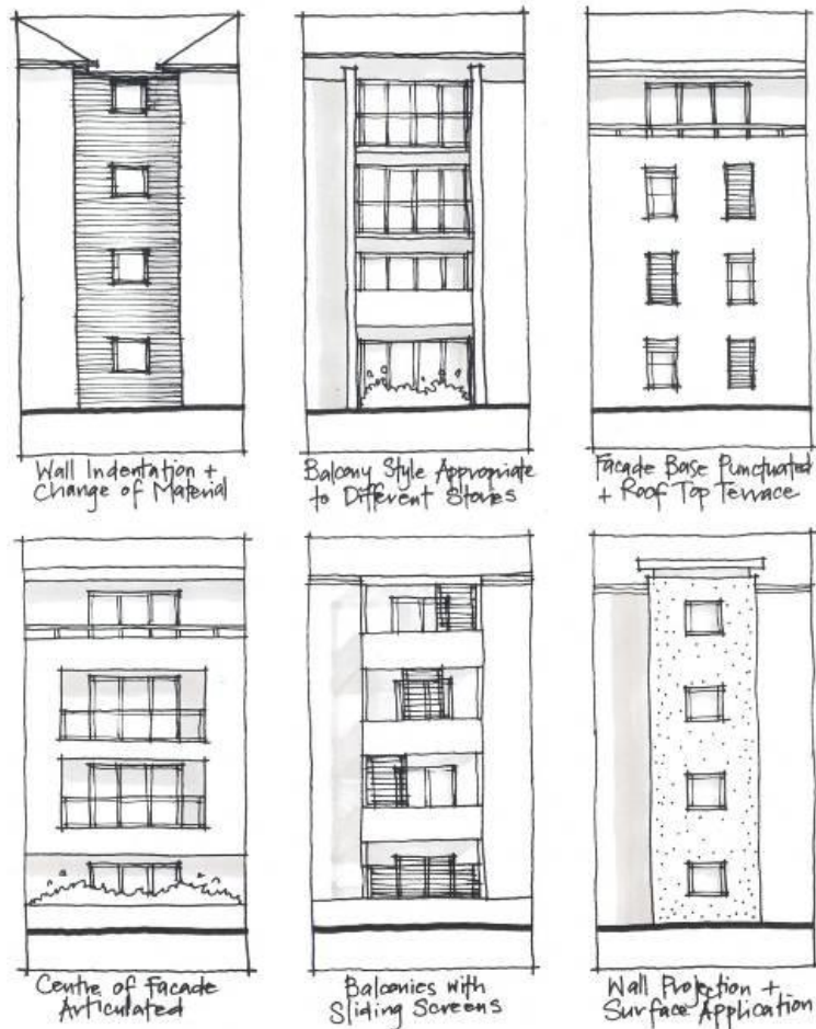
Figure 5 Examples of possible multi-storey articulated façades
