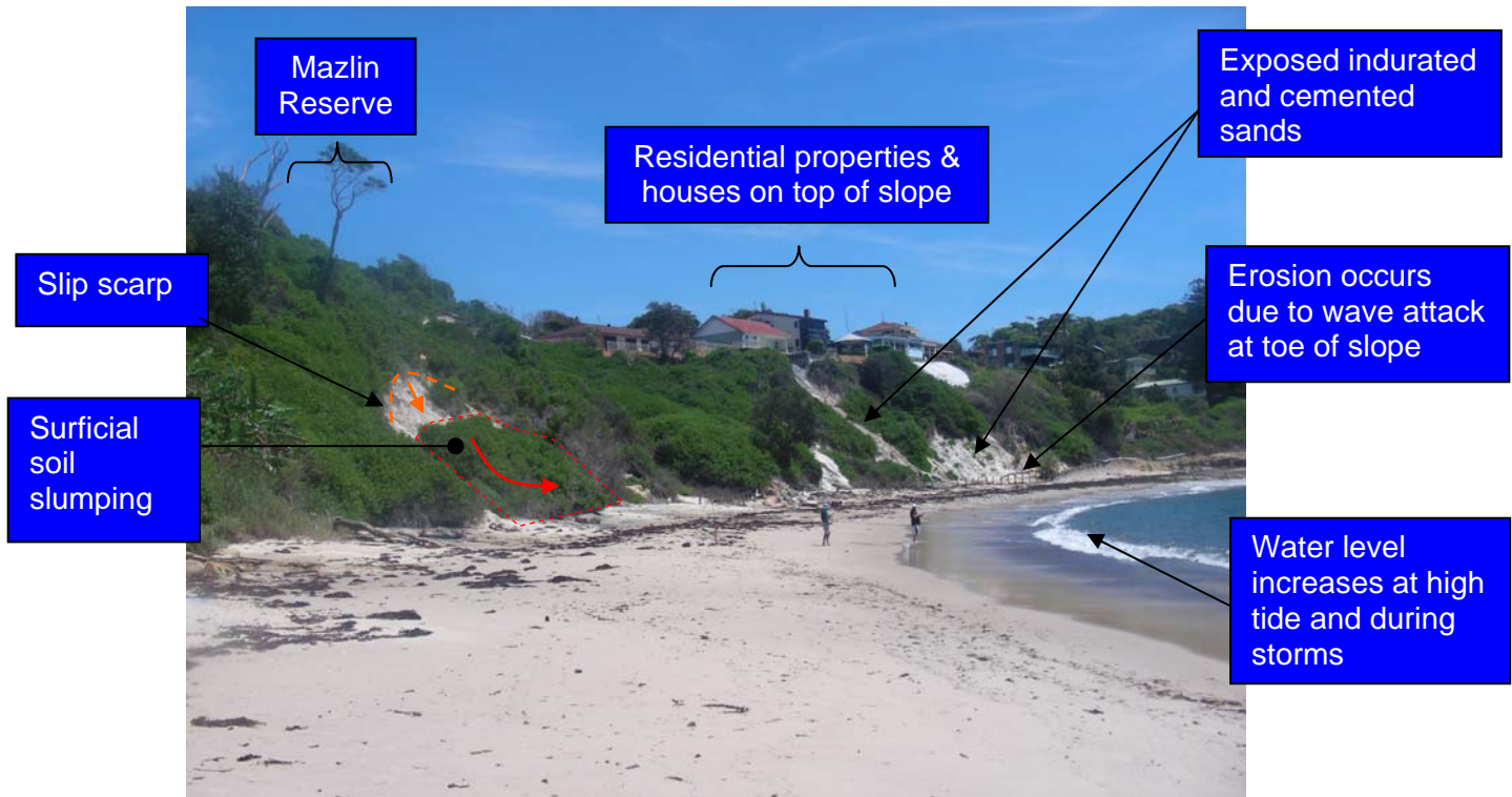
P1: Mechanism A – Indurated Sands. Map Area G11: Toe erosion & progressive surficial soil slumping.
