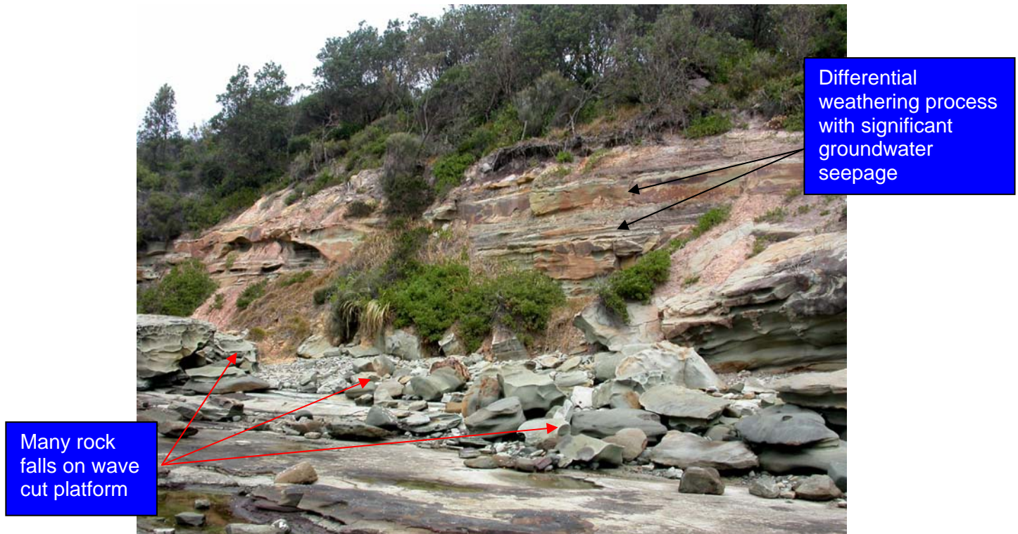
P5: Mechanism C – Rock Block / Differential Weathering. Map Areas G2 / G3: Sandstone rock falls due to ongoing differential weathering of claystone / softer bands within Patonga Claystone.
