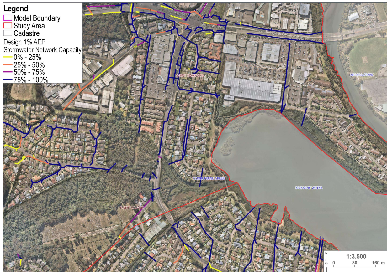
Figure 8-8 Stormwater Network Capacity at West Gosford
