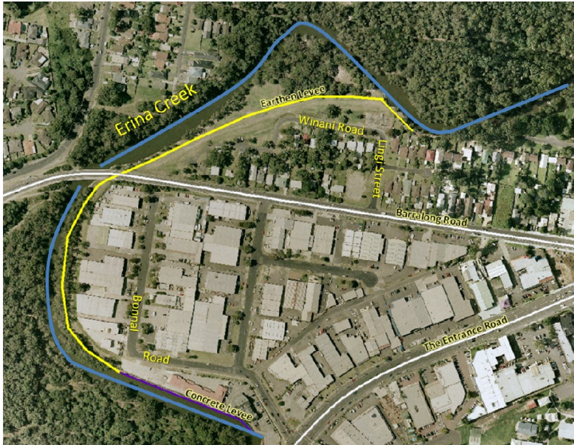
Photograph 1: Earthen and concrete levees close to Barralong Road
