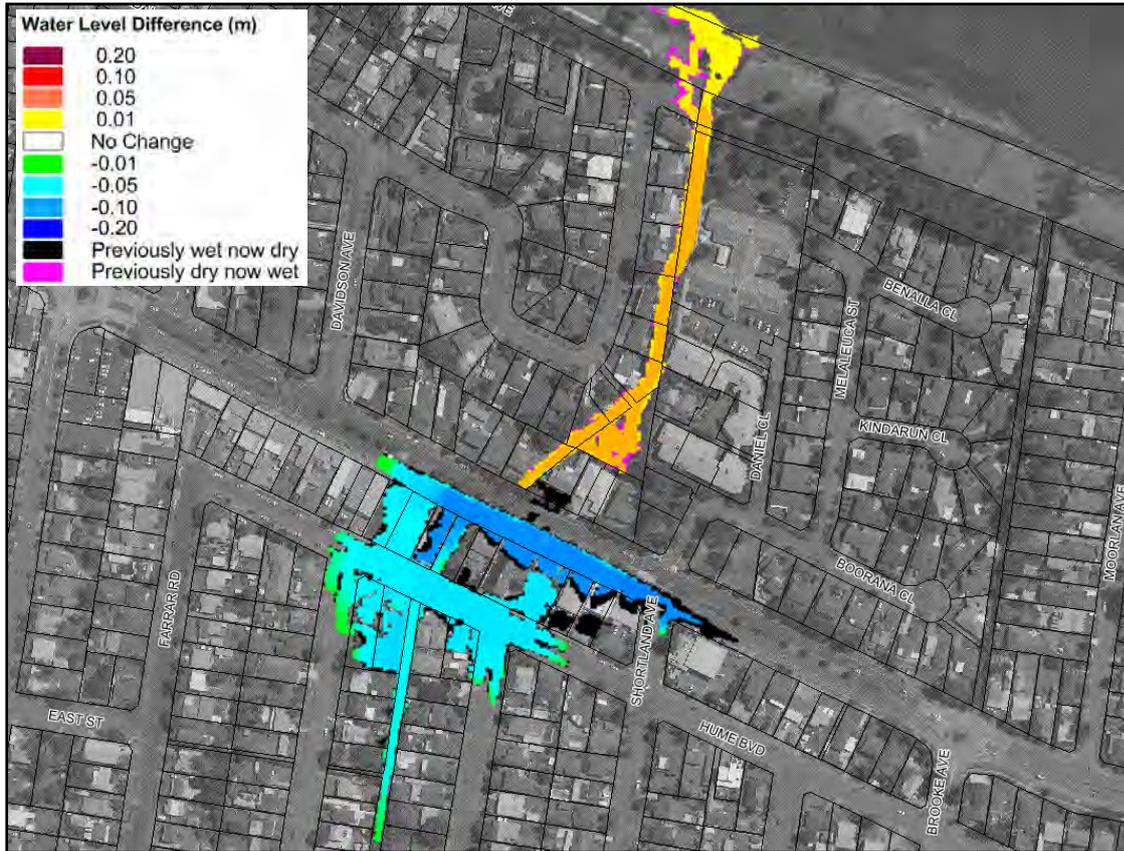
Plate 20 Peak 20% AEP Flood Level Difference Mapping with Culvert Upgrades between Hume Boulevard and Wyong Road
