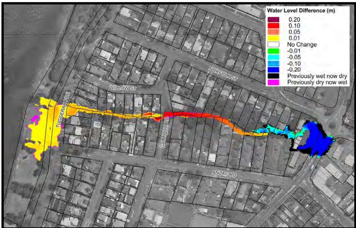
Plate 22 Peak 20% AEP Flood Level Difference Mapping with Culvert Upgrades between The Entrance Road and the rear of The Reef Resort Motel
