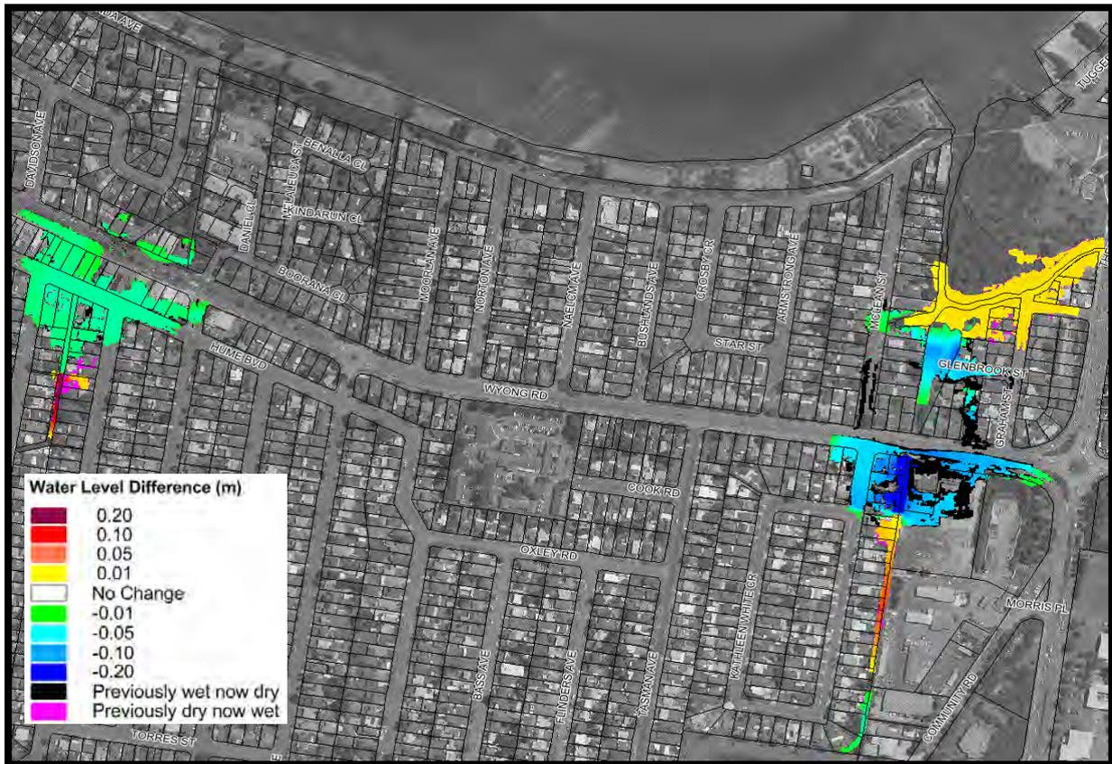
Plate 17 Peak 1% AEP Flood Level Difference Mapping with Blockage Control Structures
