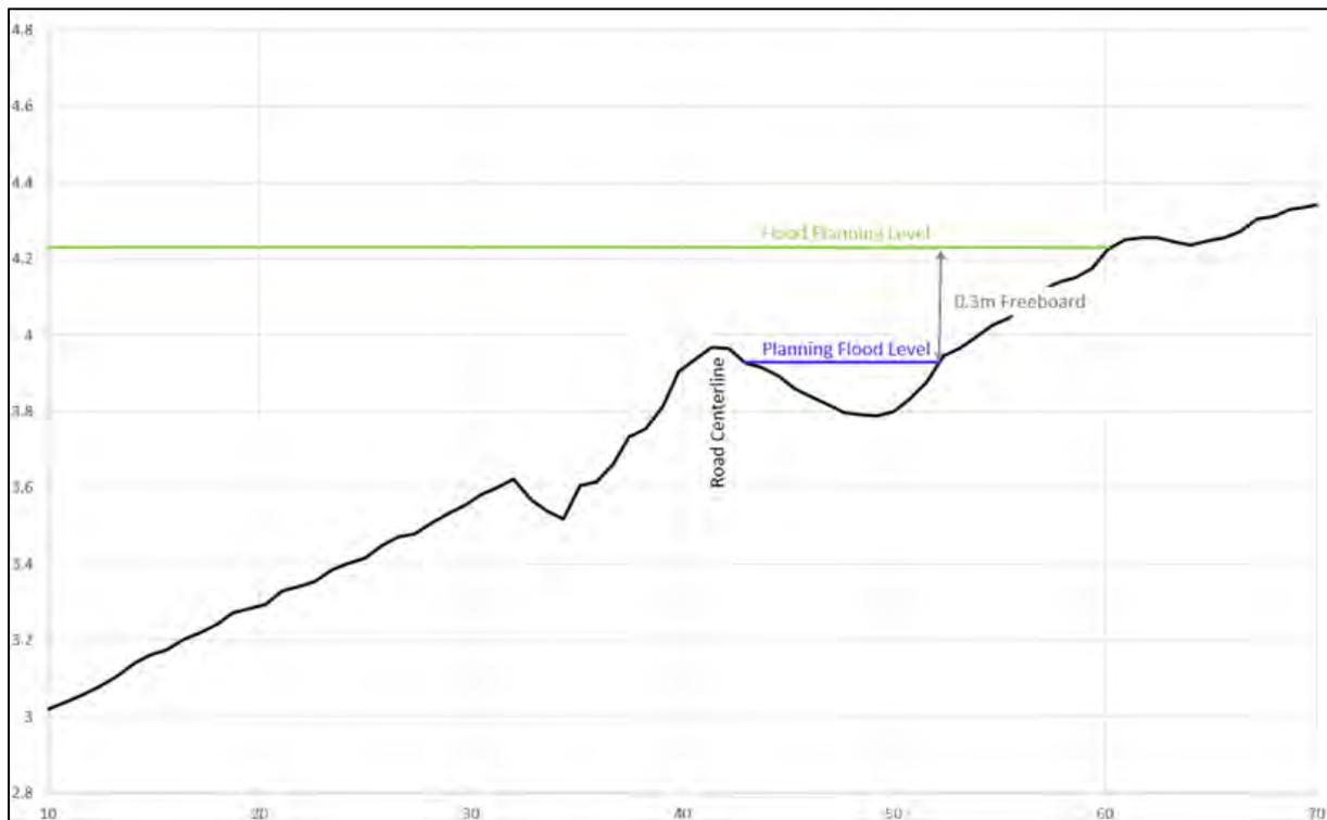
**Plate 13** Example of inappropriate FPL/FPA in urban catchment
