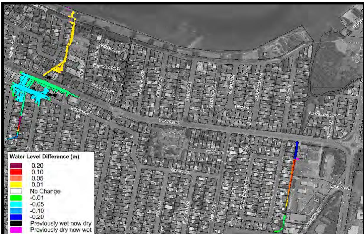
Plate 16 Peak 20% AEP Flood Level Difference Mapping with Blockage Control Structures
