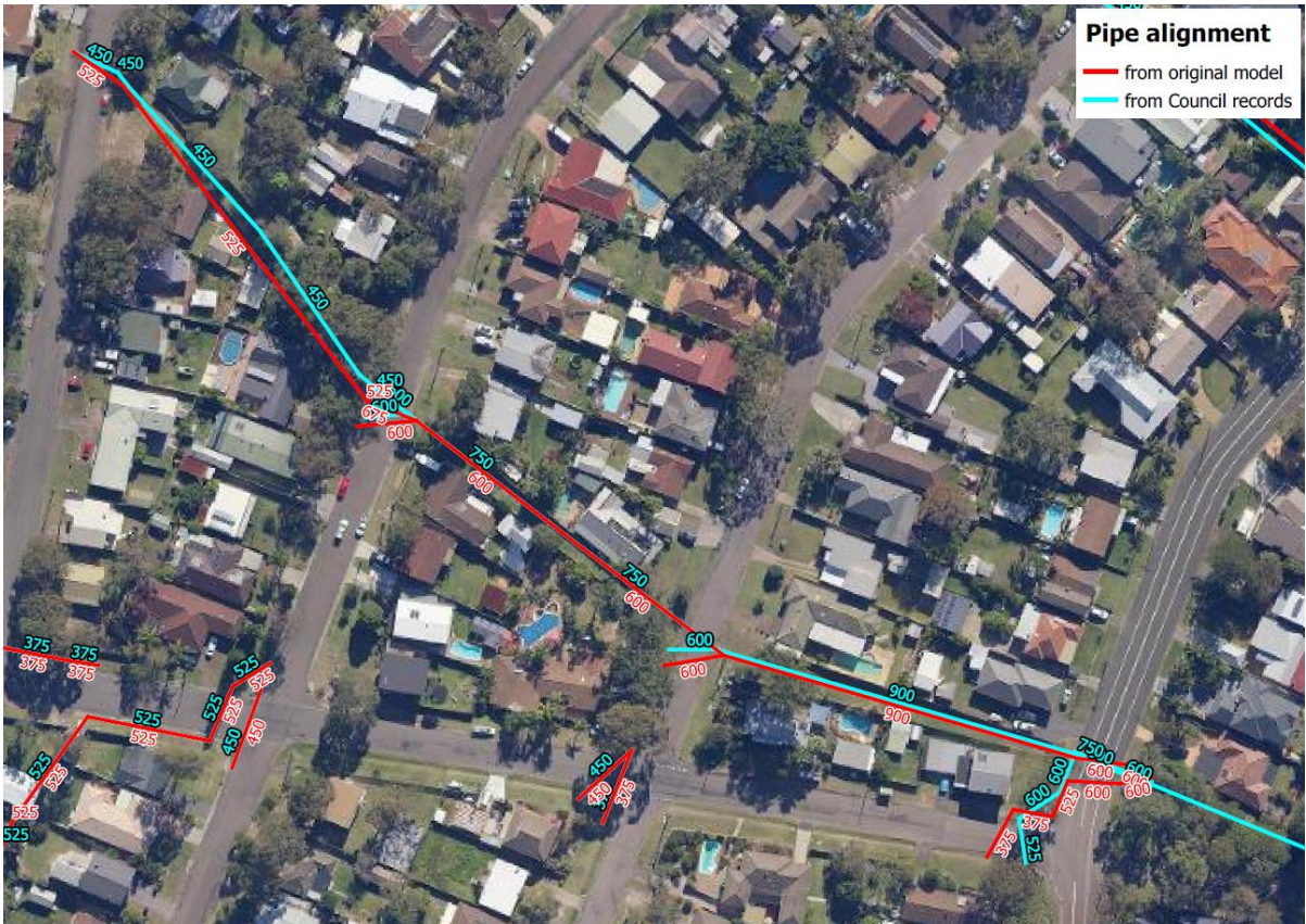
Figure 6.14 – Minor Discrepancies between Council and Modelled Data (Diameters displayed along pipes are in mm) Top Budgewoi; Bottom: Halekulani Aerial source: NSW Spatial Services
