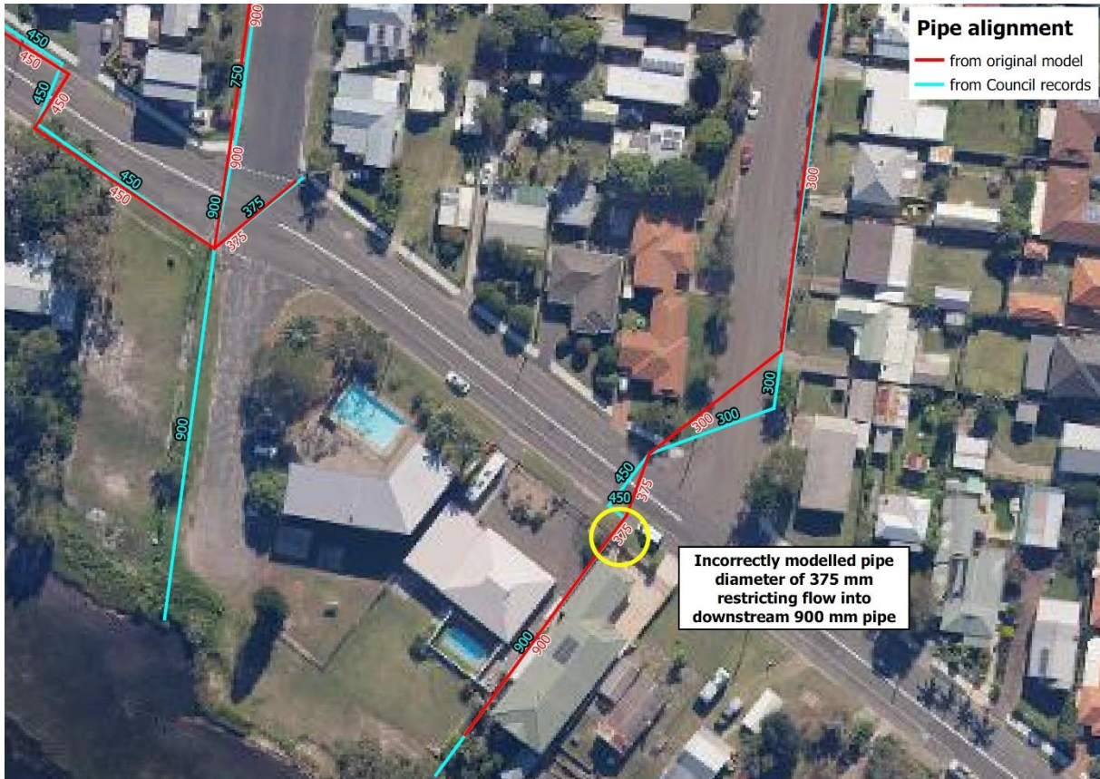
Figure 6.15 – Location of incorrect pipe size in Moss Avenue, Toukley (Diameters displayed along pipes are in mm)
