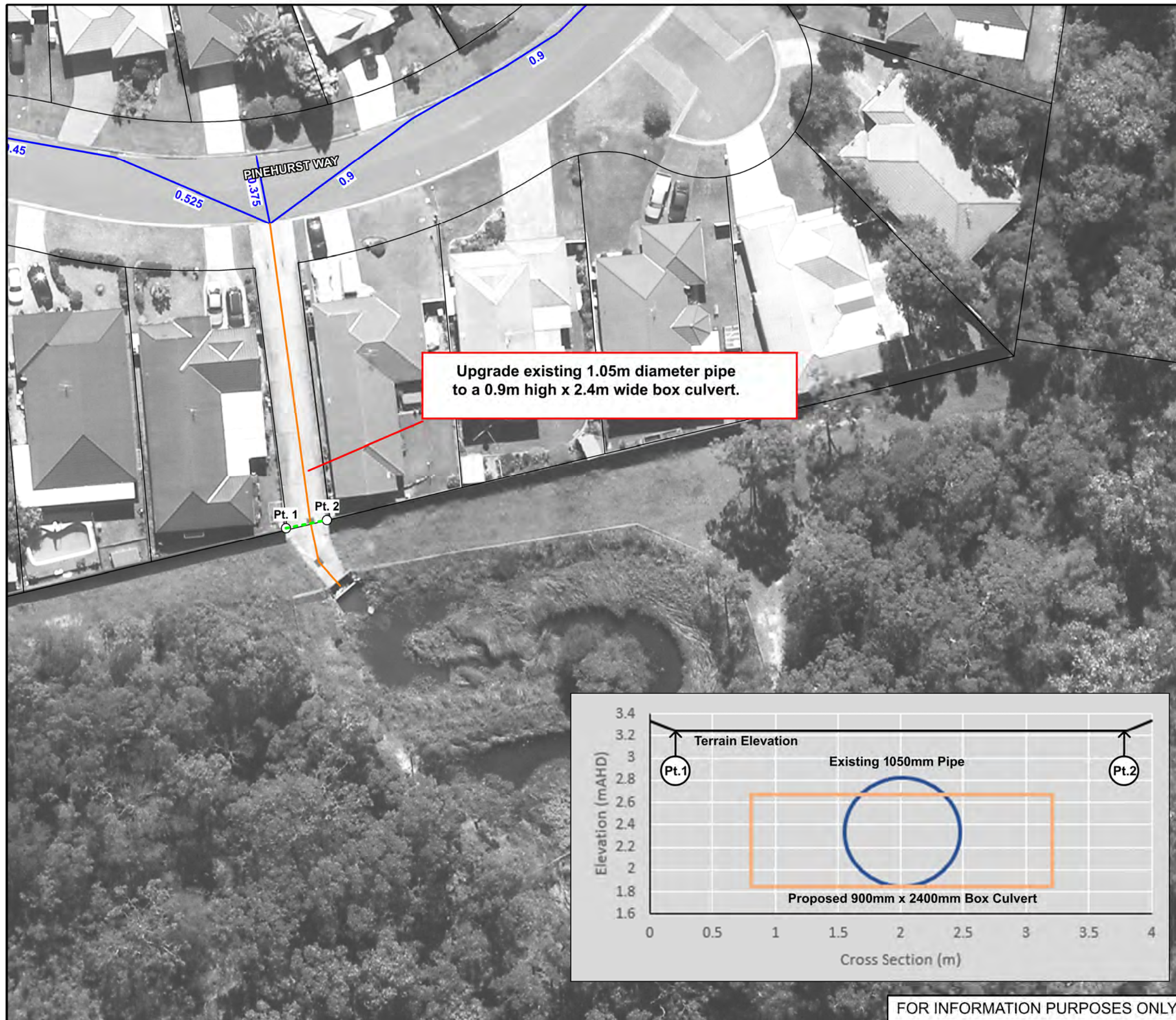
Figure 25: Concept Design for the Pinehurst Way Stormwater Upgrade (FM3)
