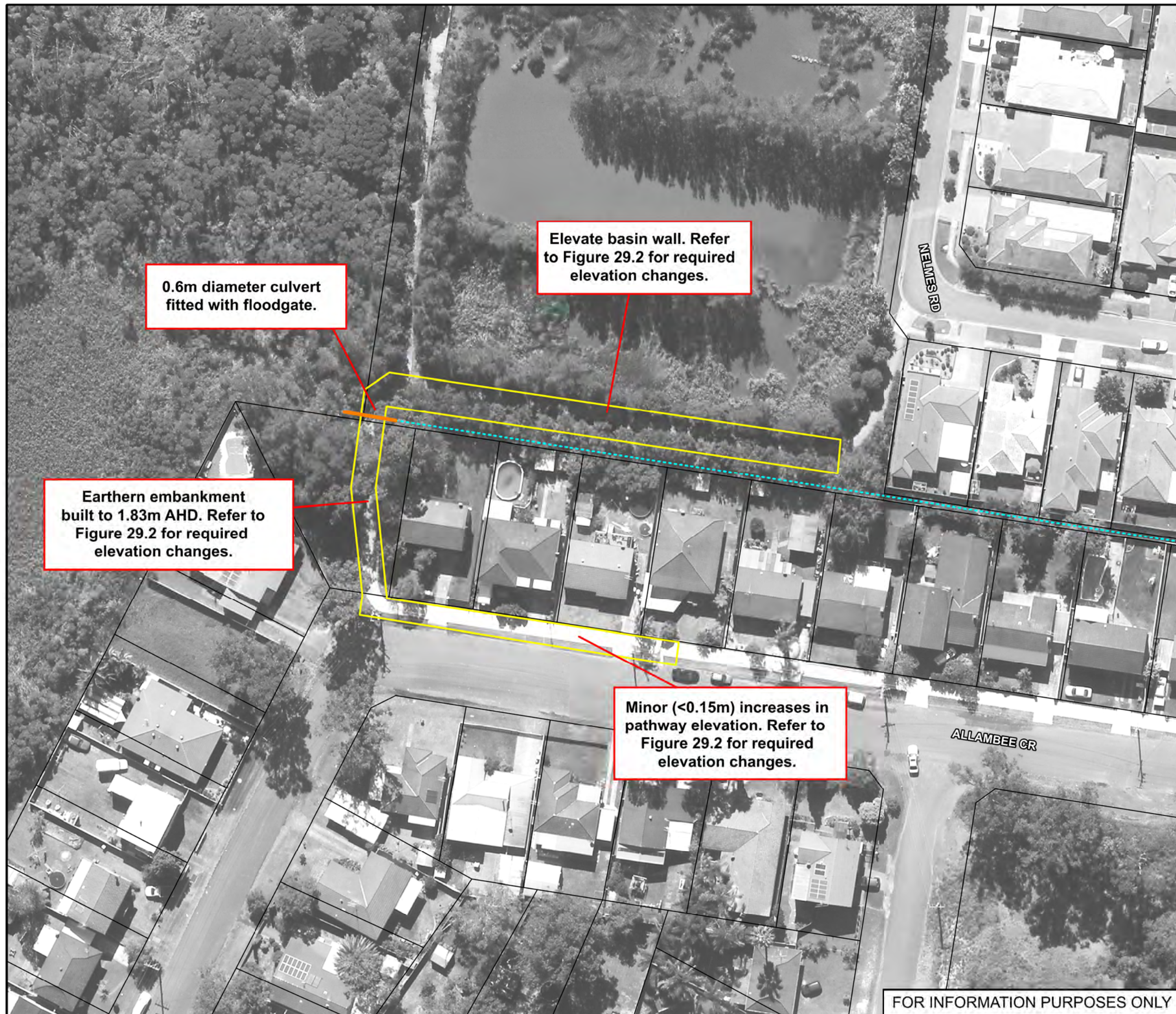
Figure 29.1: Concept Design for the Allambee Crescent Channel Modifications (FM7)
