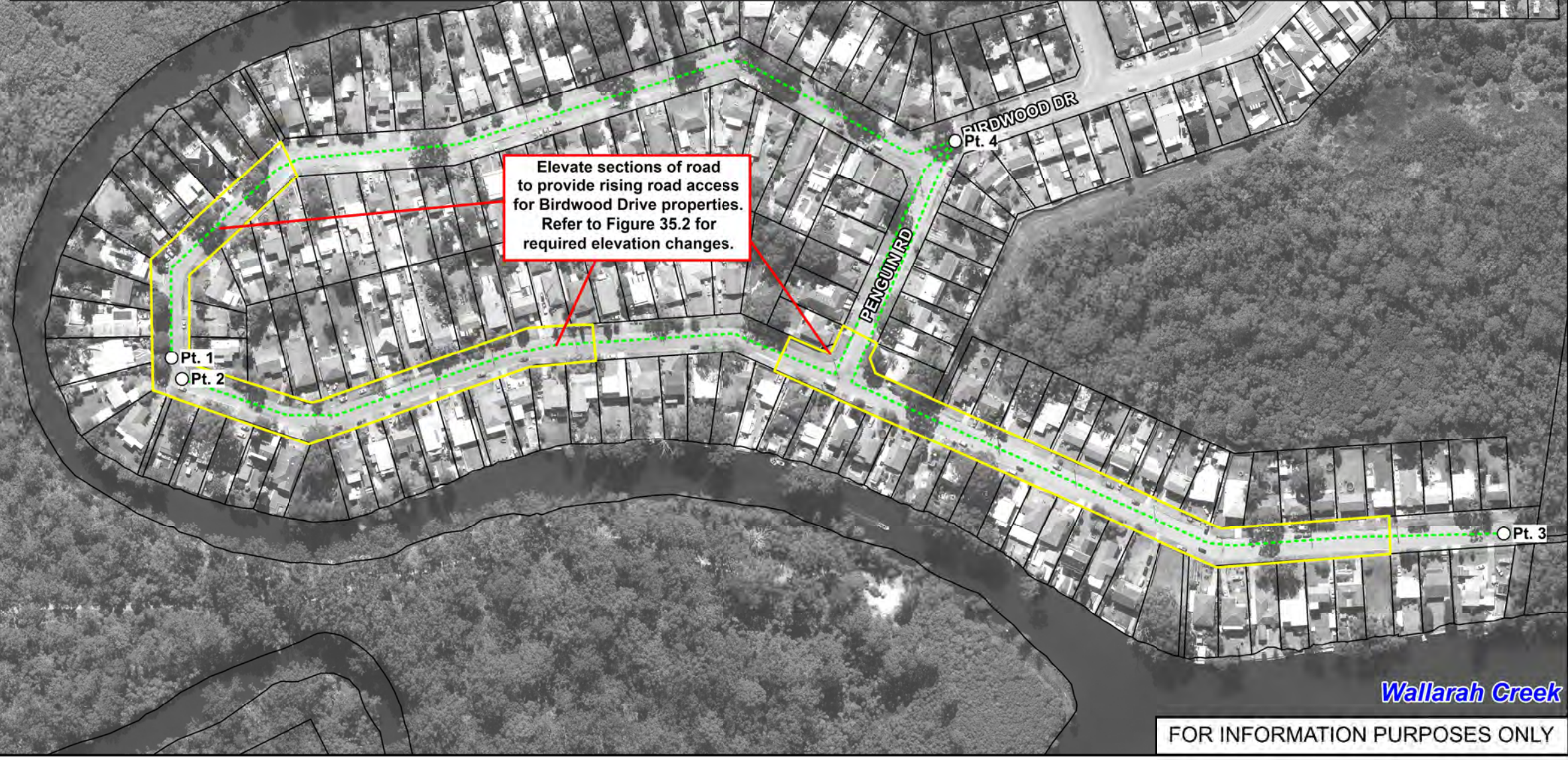
Figure 35.1: Concept Design for the Upgrade of Birdwood Drive (RM6)
