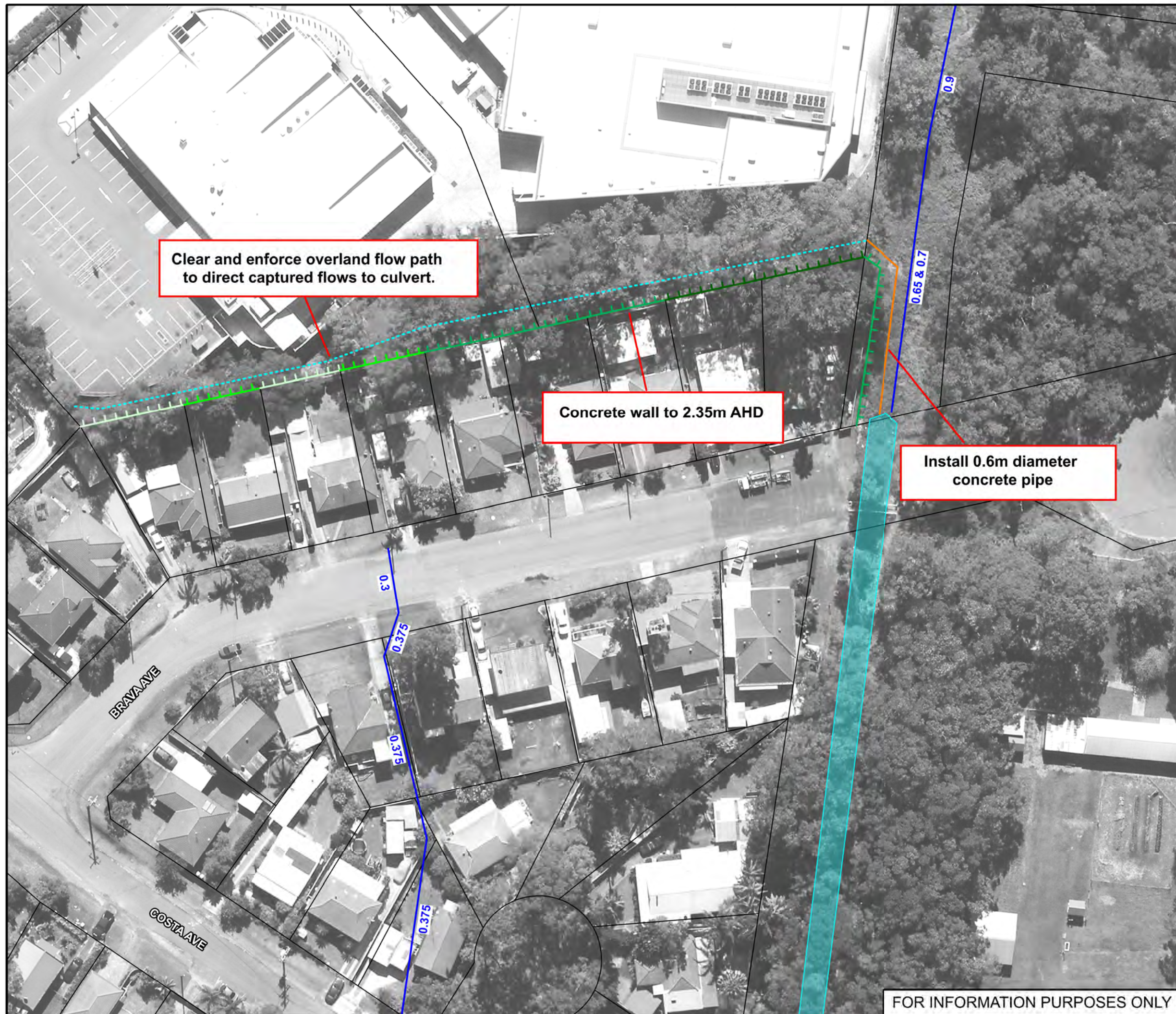
Figure 26: Concept Design for the Brava Avenue Floodwall and Drainage Upgrades (FM4)
