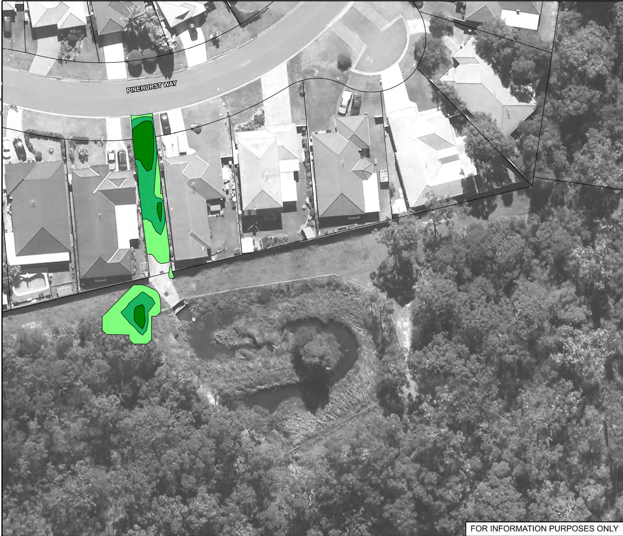
Figure 32.2: Concept Design for the Pinehurst Way Flow Path Reshaping (FM10)
