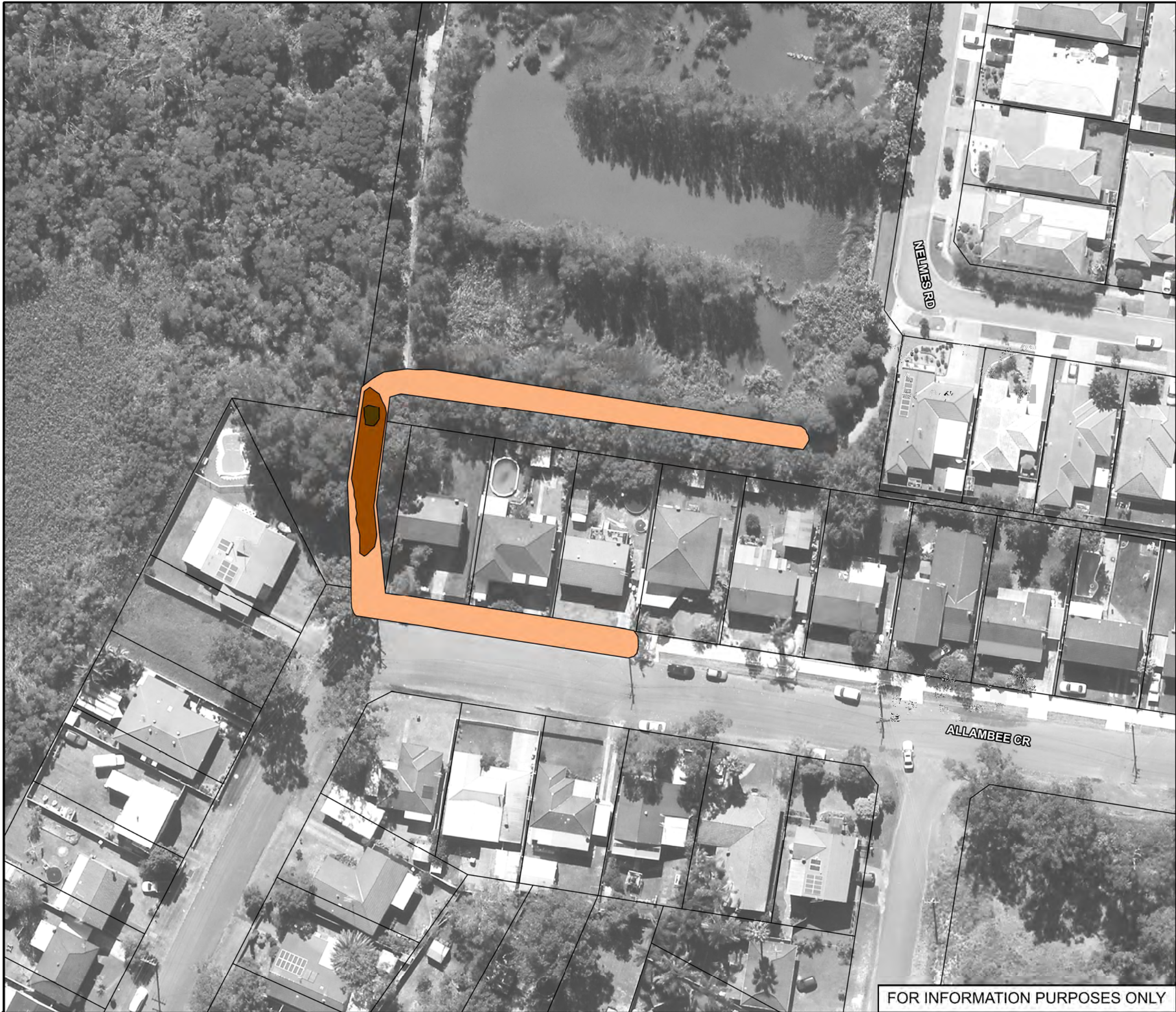
Figure 29.2: Concept Design for the Allambee Crescent Channel Modifications (FM7)
