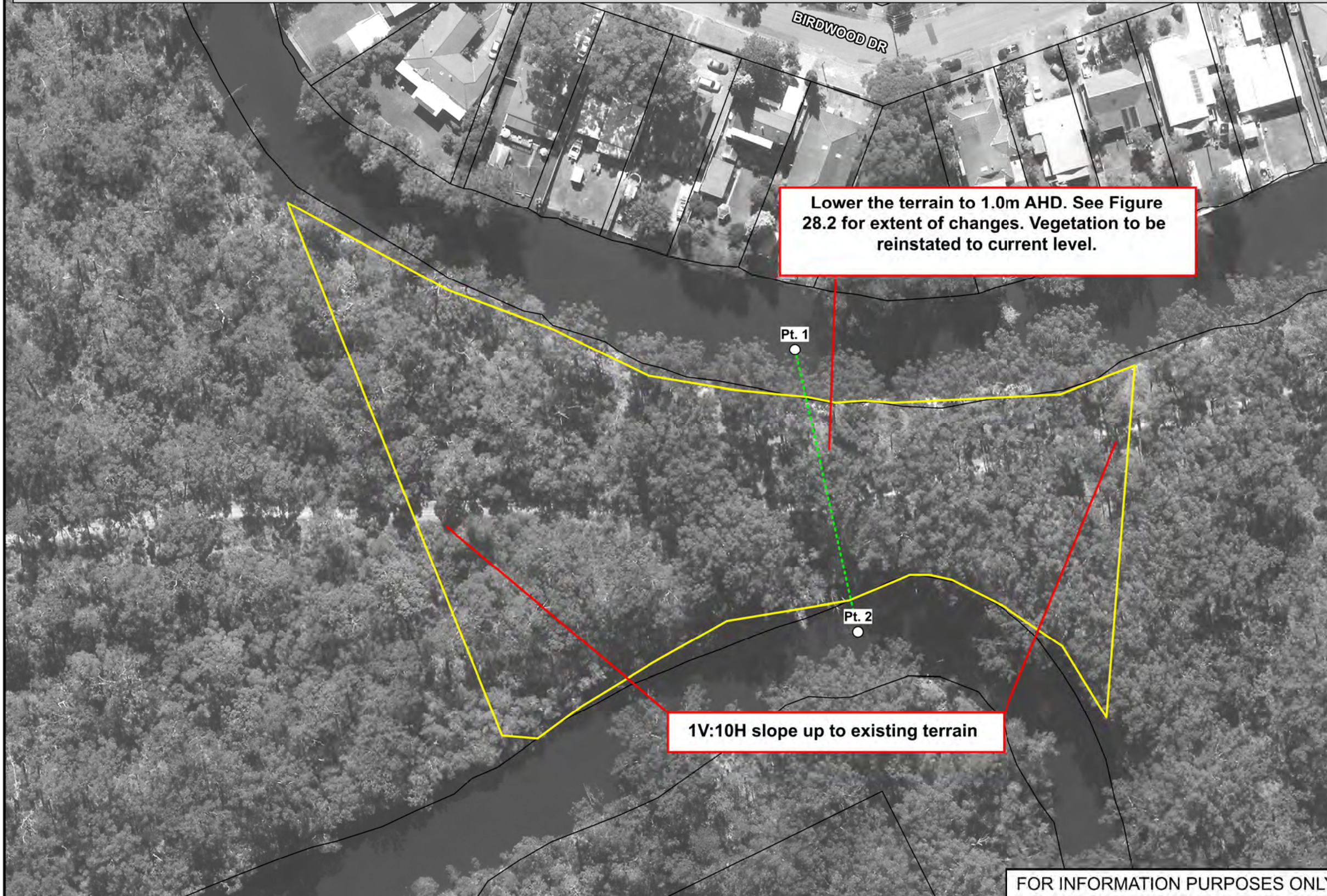
Figure 28.1: Concept Design for the Spring Creek High Flow Bypass (FM6)
