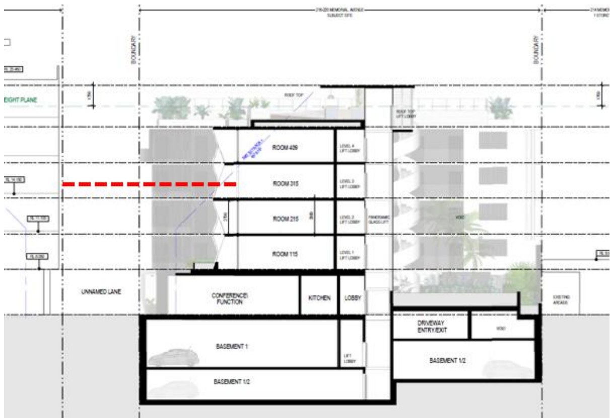
Figure 14 – Proposed section showing distance achieved between proposed hotel rooms and the existing Atlantis development (15m) (dashed in red)
