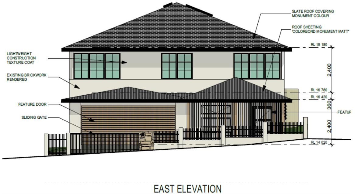
Figure 4: The proposed eastern (street) elevation
