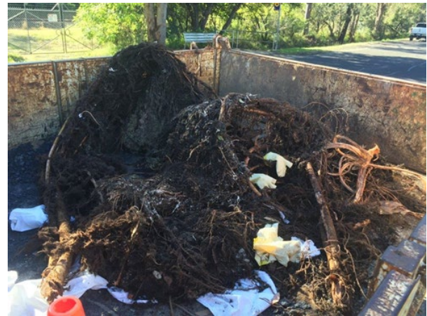
Figure 4: Tree roots and other solids removed from a sewer main in Council's sewer system
