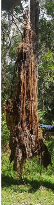
Figure 1: Root mass removed from a manhole in Council's sewer system
