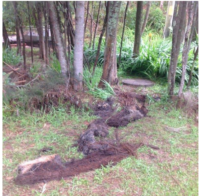
Figure 2: Root mass removed from a sewer main in Council's sewer system
