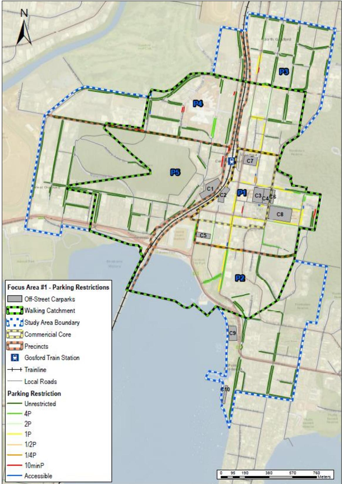
Figure 2.5: Focus Area #1 – Gosford: Kerbside Parking and Off-Street Parking Locations
