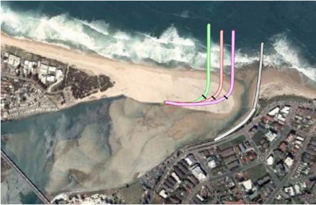
Figure 3. Cardno modelled training wall scenarios (2013)
