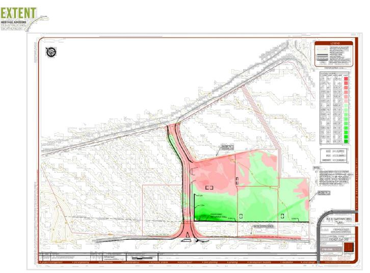
Figure 37. A Bulk Earth Working Plan showing the percentage of area to be stripped and refilled to make level ground. The plan also includes areas to be replanted (source: ADW Johnson, Bulk Earth Working Plan, Drawing No.190427-DA-005).
