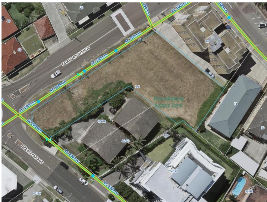
Figure 14: Water servicing arrangements
