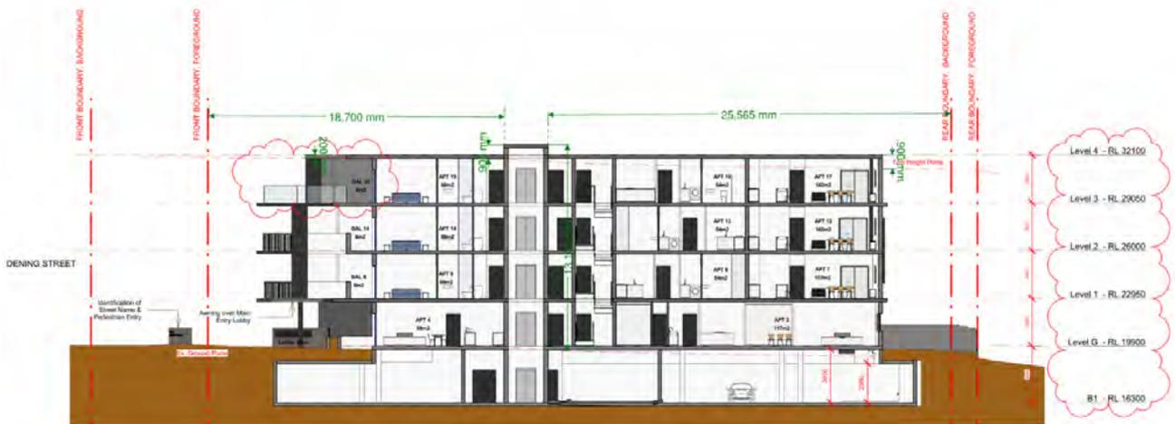
**Above: Section showing height breach**
