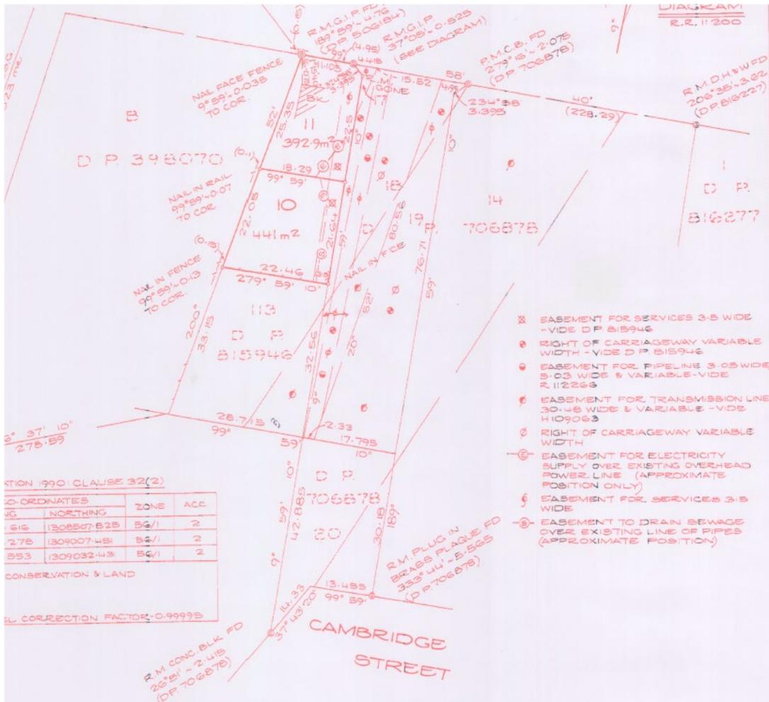
**Figure 3 - Extract from DP 875531 showing easements and rights of carriageway**
