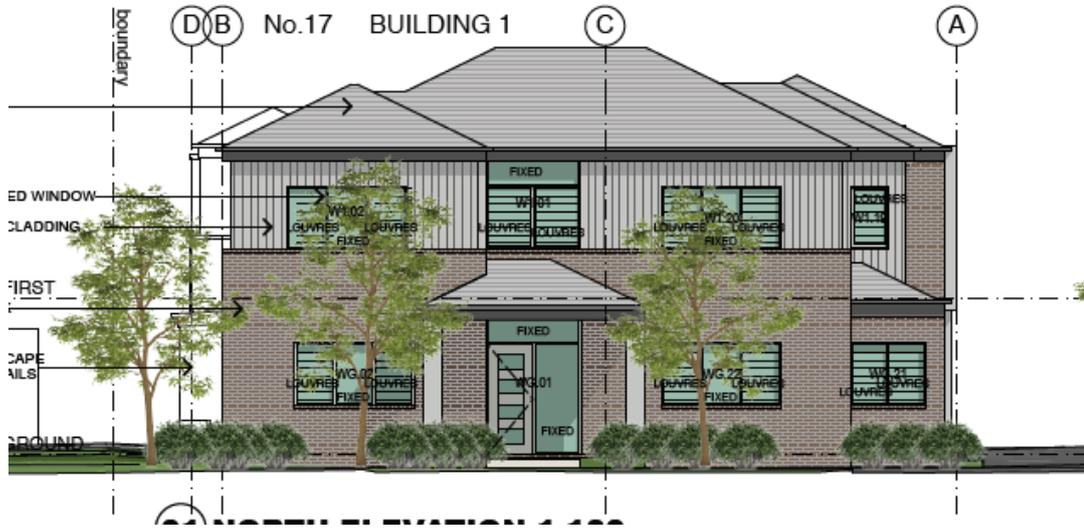
**Figure 11 - Proposed presentation of building 1 (north elevation)**
