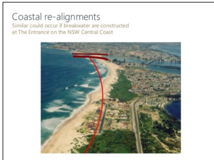
Figure 4 - Training walls at The Entrance would likely cause coastal realignment leading to erosion at Curtis Parade (slide 10 from Neilson presentation)
