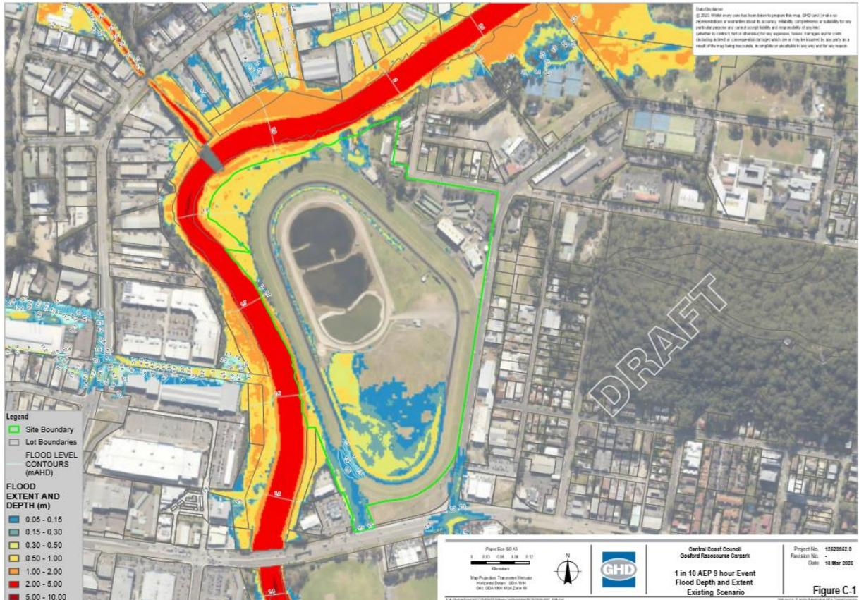
Figure 6 demonstrates the existing implication of a 1 in 10 AEP flooding effect on the Racecourse. As demonstrated the Racecourse floods on its southern part of the site and an on-grade carpark without any adjustments to its base height level would inundate the Racecourse with flood waters.
