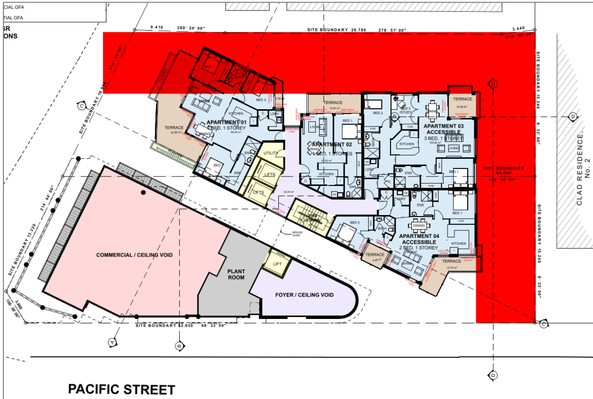
Figure 9 – Areas on non-compliance with half of ADG building separation levels 1 to 4 (6m)
