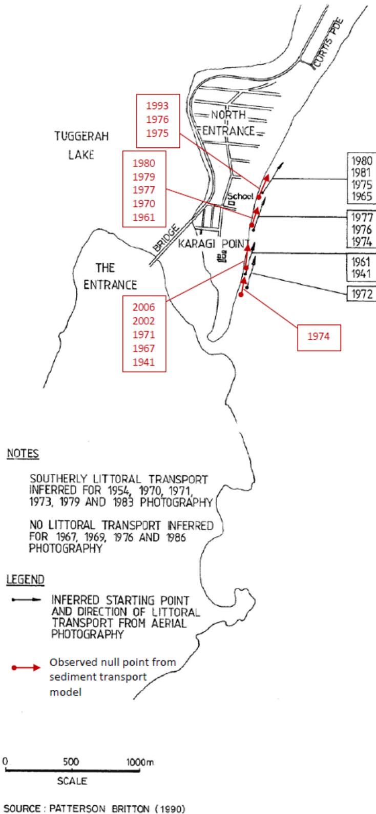
Figure 5.5 Locations of null point observed from sediment transport model compared with Worley Parsons (2008).
