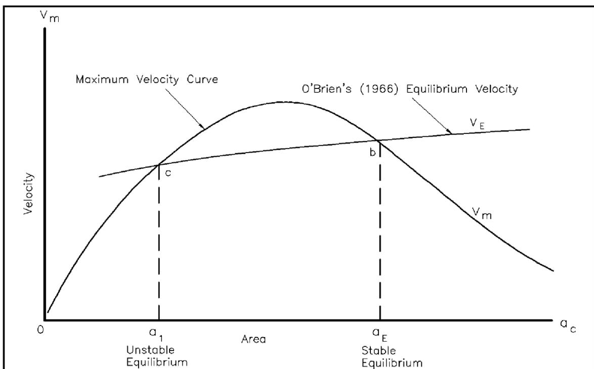
Figure 6.1 – Escoffier (1940) curve, maximum and equilibrium velocities versus inlet cross-sectional area (C.E.M., Chap. II-6)
