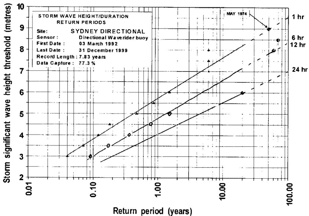
Figure 4.5 – Storm wave height duration recurrence (Lord & Kulmar, 2000)
