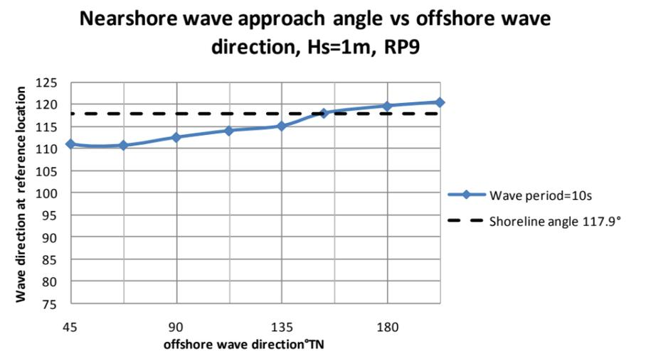
Figure 4.7 – Nearshore swell wave approach angle vs. offshore wave direction, Reference Point 1-9
