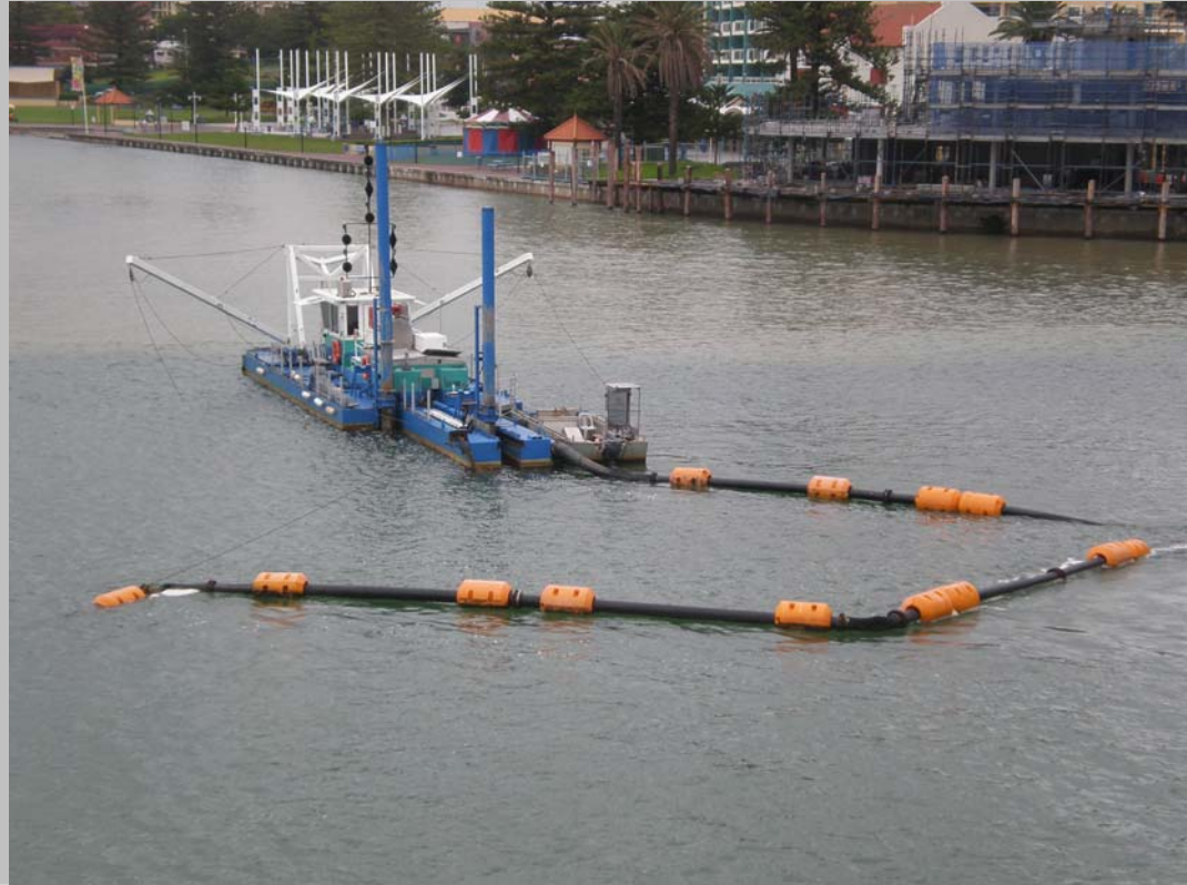
Photo 1 - Wyong Shire Council's Cutter Suction Dredge
