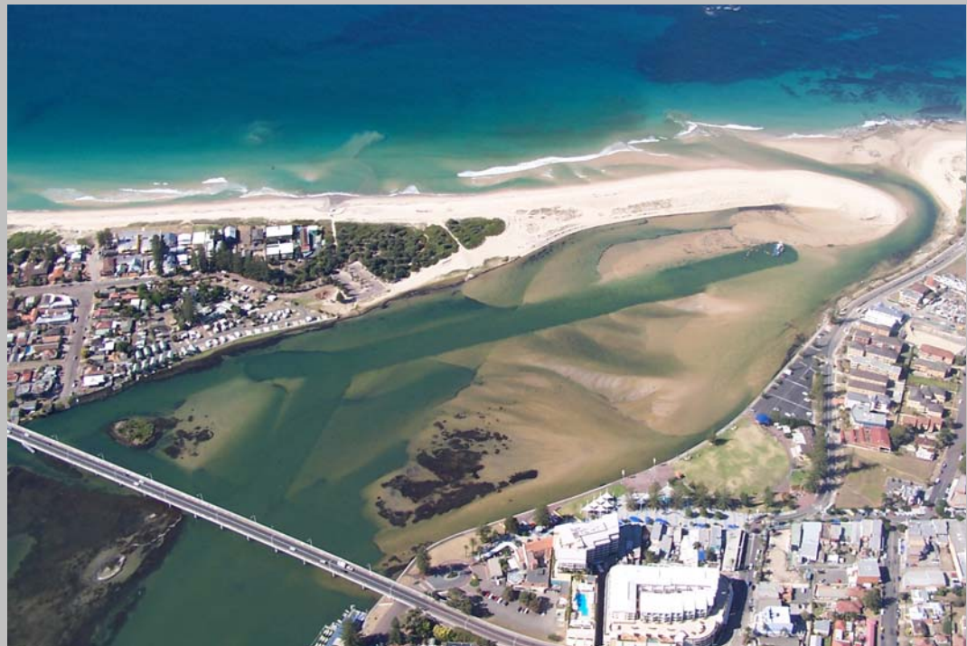
Photo 2 - The Entrance Channel – typical alignment of dredged channel with dredging commencing at the upstream extremities such that dredging effort is enhanced by the ebb tide.
