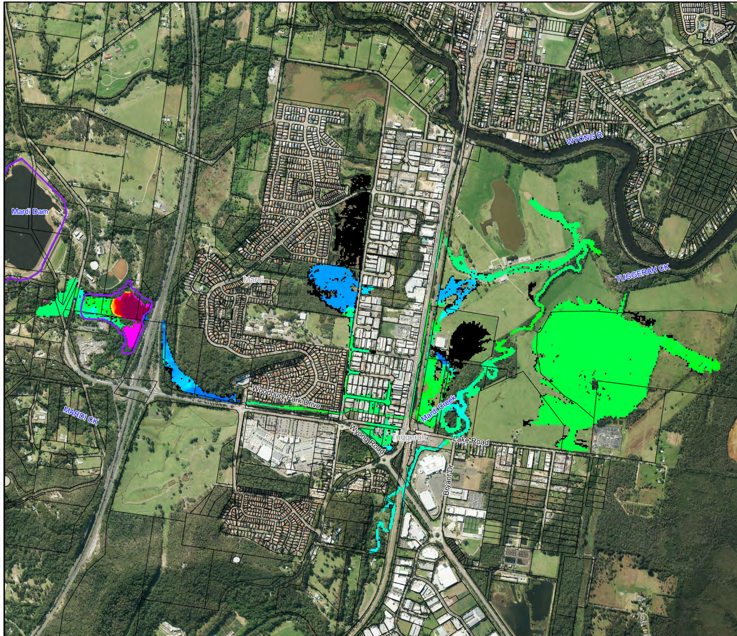
Figure B4: Flood Level Difference Mapping for the 20% AEP Flood with Mardi Creek Detention Basin
