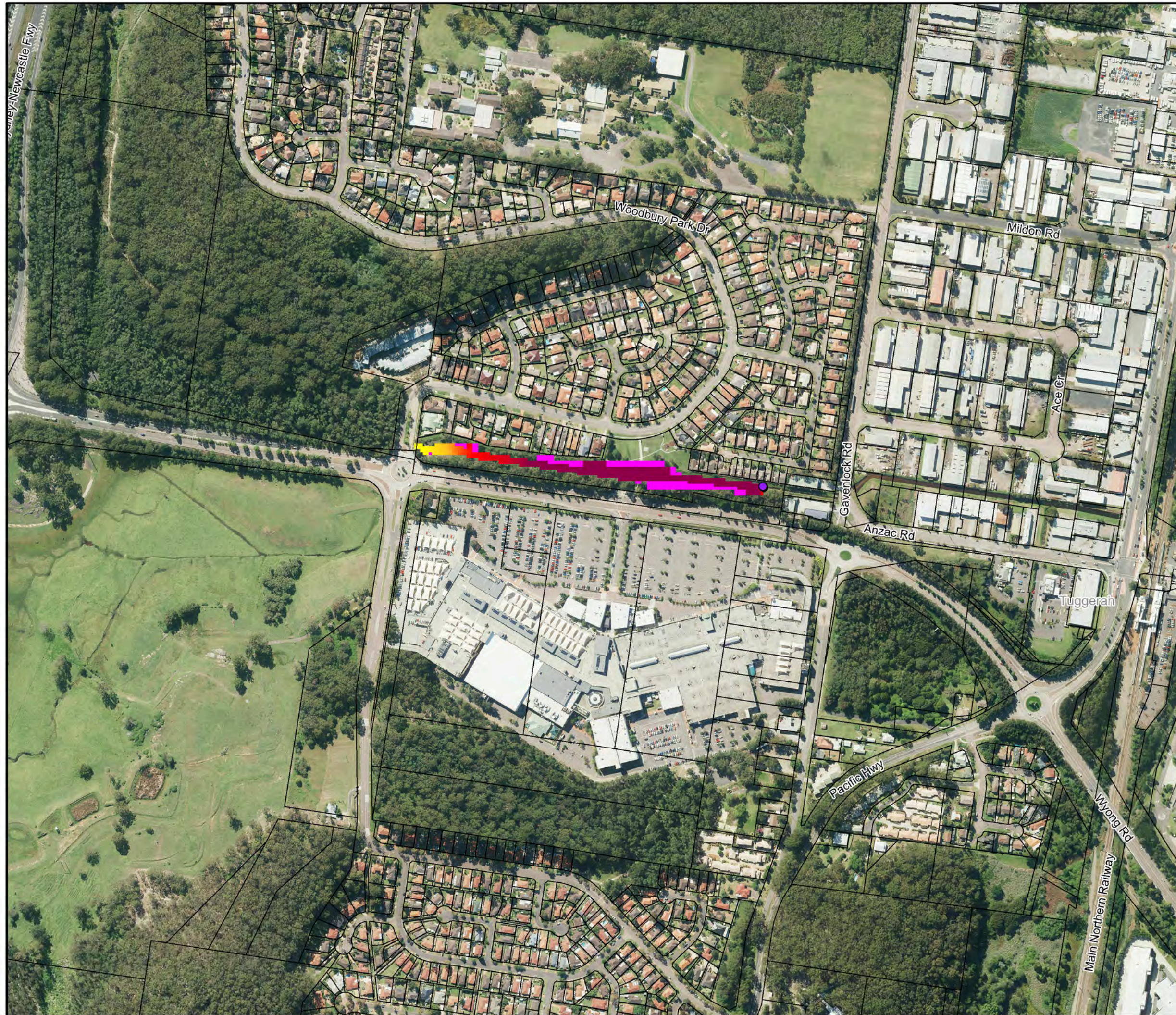
Figure G4: Flood Level Difference Mapping for the 20% AEP Flood with Debris Control Structures
