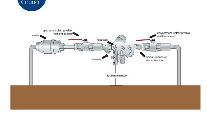
Typical installation of Backflow Prevention Device
