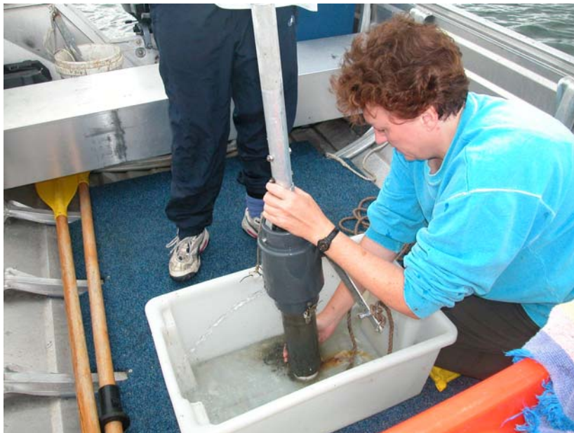
Plate 1. Field sampling for biomass of benthic microalgae showing the sediment corer being lowered into the water (upper photo) and retrieval of sediment sample in perspex corer (lower photo).
