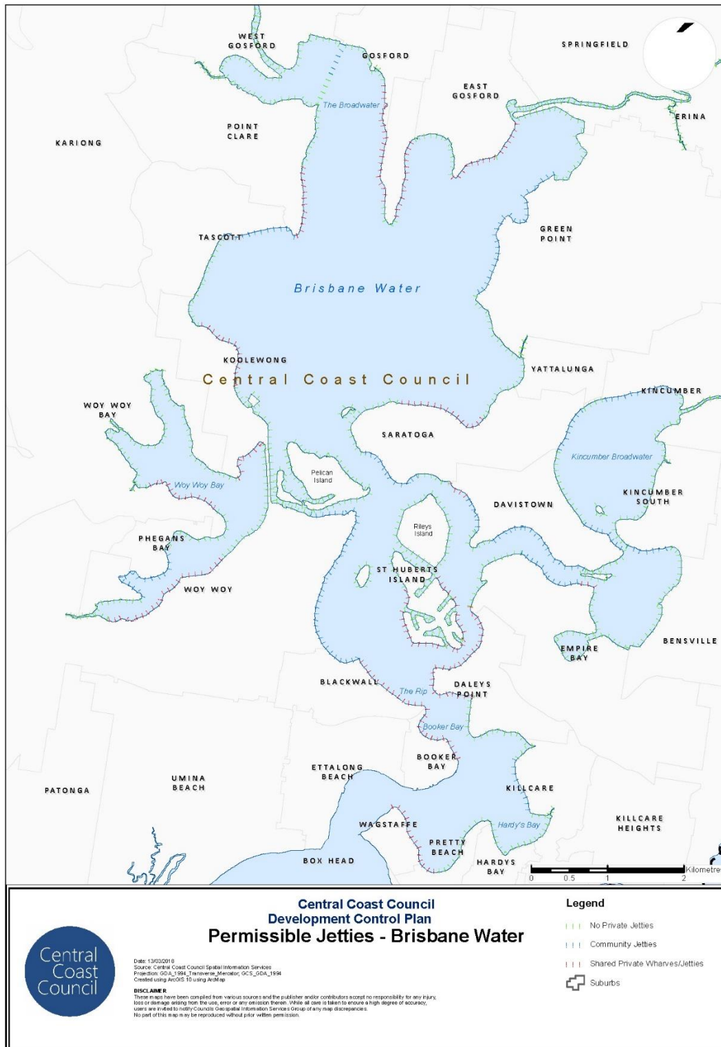
Figure 1: Permitted Wharf and Jetty Types – Brisbane Water
