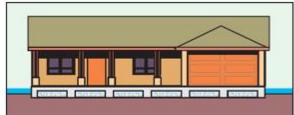
Raising the slab on waffle pods is effective in reducing the possibility of the house being inundated by overland flooding 4
