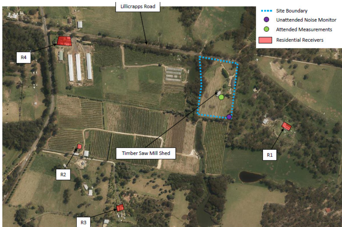
Figure 7 – Acoustic Assessment map indicating noise measurement locations.
