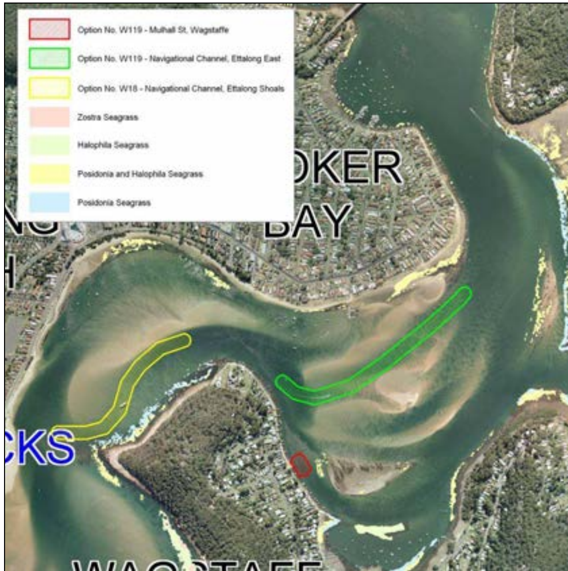
Figure 3.6: Dredging Options and Seagrass Distribution within the Ettalong/The Rip CLAM Area
