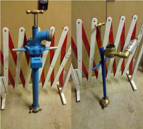
Figure 1: 63mm (3-lug connection) and 25 mm (2-lug connection) metered standpipes
