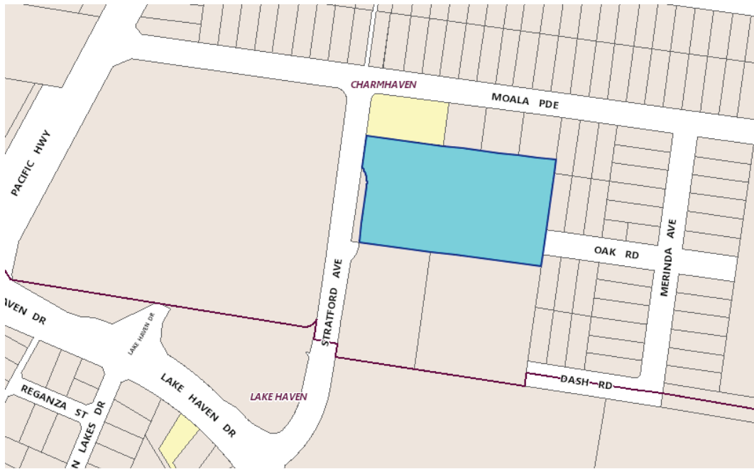
Figure 2 – Cadastral plan showing road network in vicinity of site (note: the portion of Stratford Avenue fronting the development site is currently unformed)
