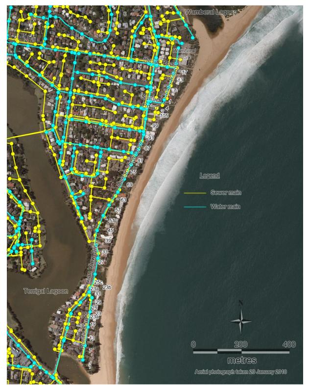
Figure 9: Sewer and water infrastructure in and adjacent to study area
