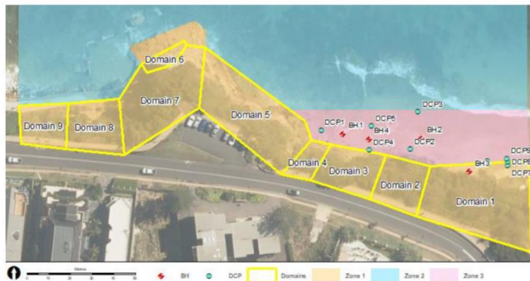
Figure 5: Layout of geologic domains
