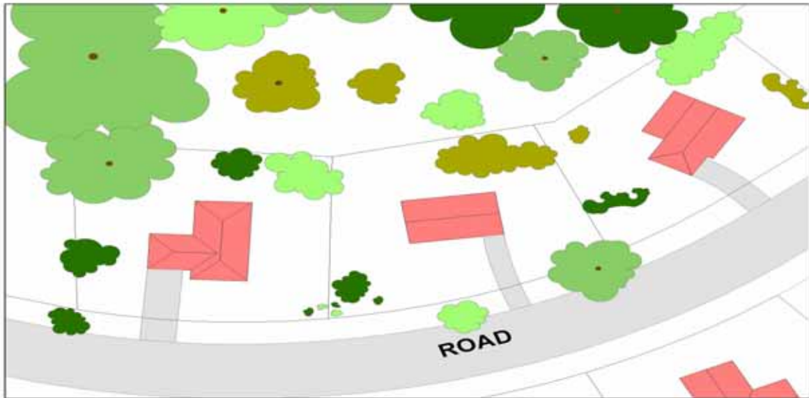
FIGURE 7: LARGE IRREGULAR SHAPED LOTS PERMIT VEGETATION RETENTION, VARIOUS BUILDING FORMS AND LIMIT NEED FOR CUT AND FILL
