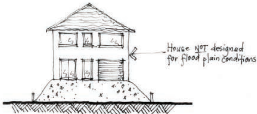
Figure 3 Inappropriate floodplain development
