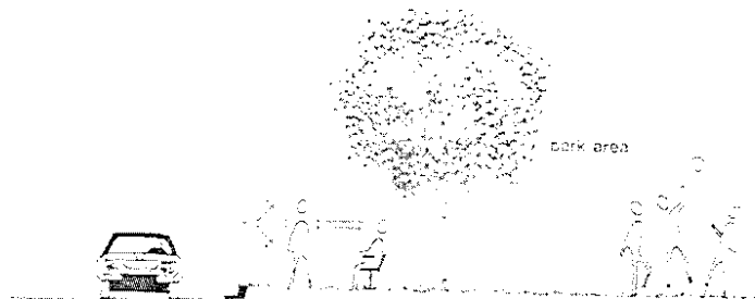
Fig. 82 Where there is a pleasant view or interesting activity, seating should not face motor traffic.
