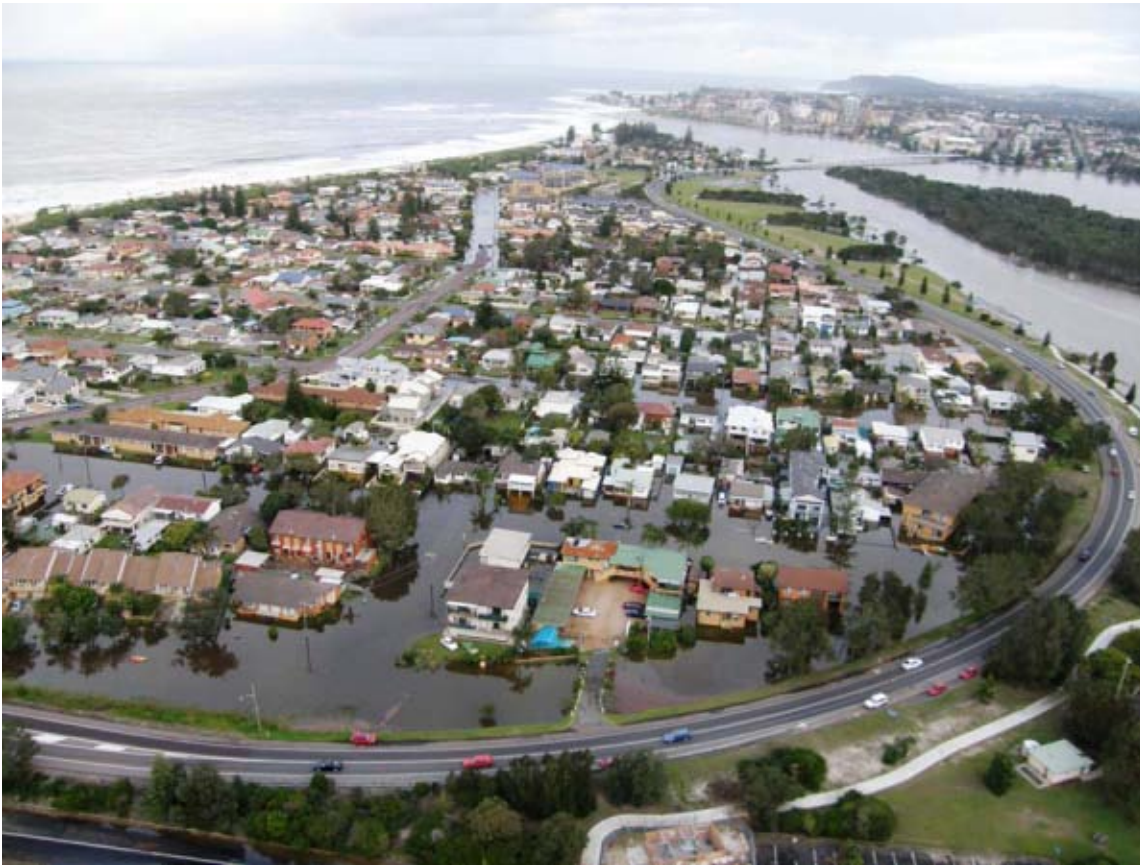
Figure 1: Aerial photo of The North Entrance inundated during the June 2007 flood event (estimated to be about a 10% AEP event).
