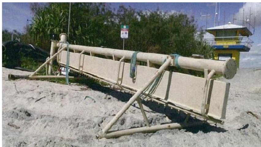
Figure 5-4 Slurry systems sand shifter
