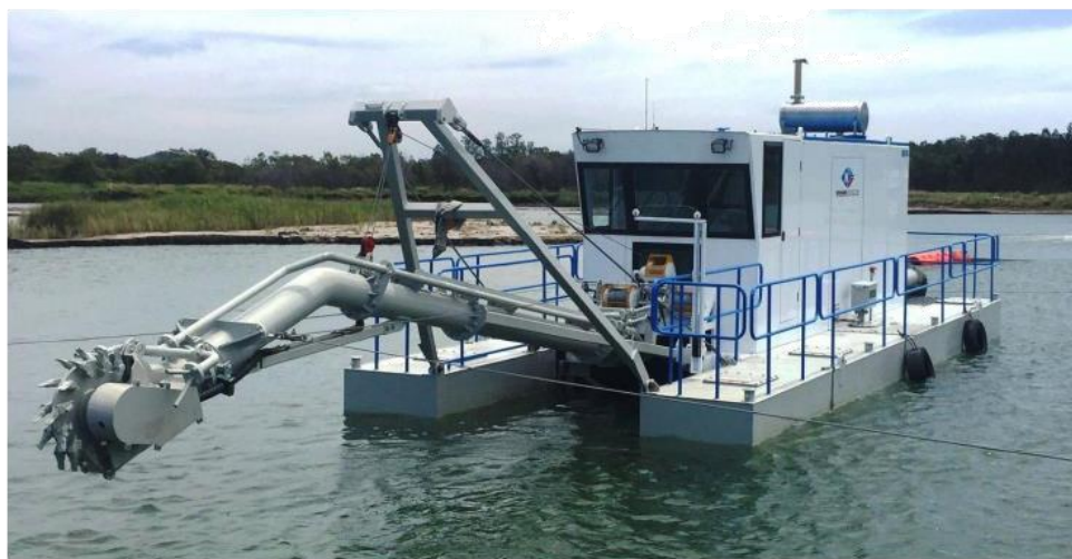
Figure 5-1 Neumann contractors cutter suction dredge
