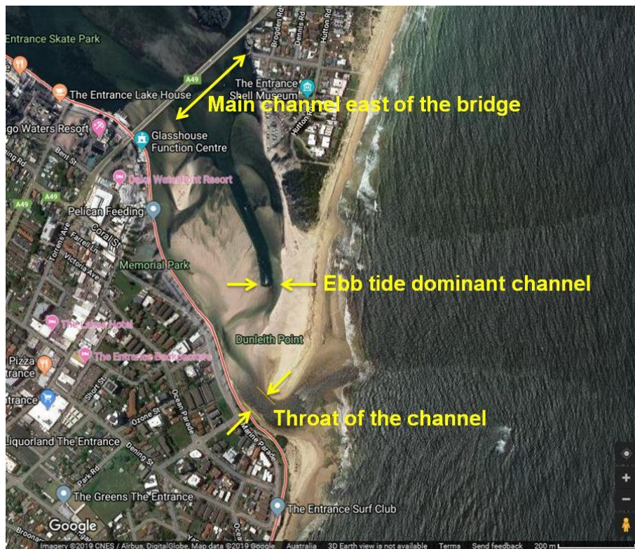
Figure 3. Key locations where triggers for dredging at The Entrance Channel are considered
