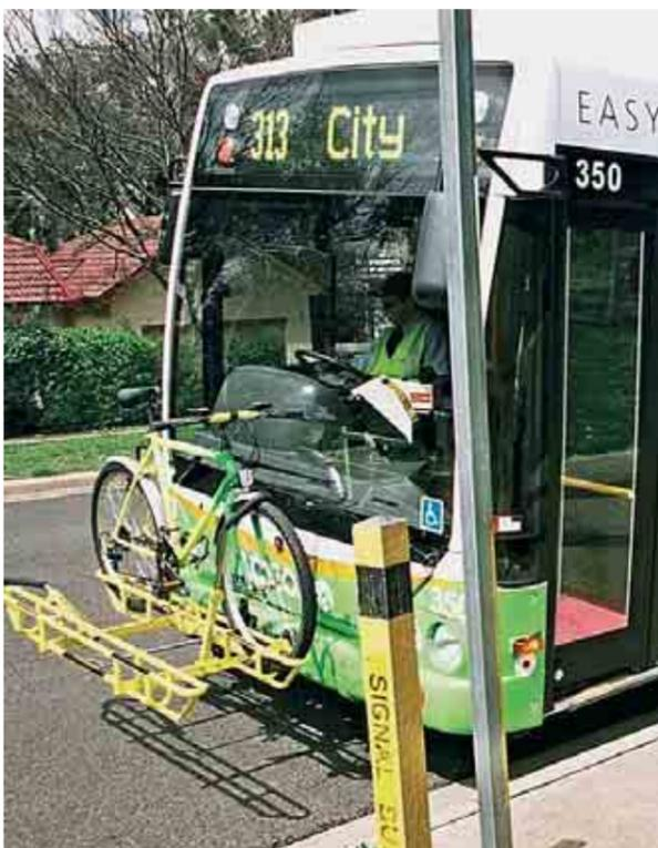
Fig 7.6.2 Example: 'Rack and Ride' facilities
