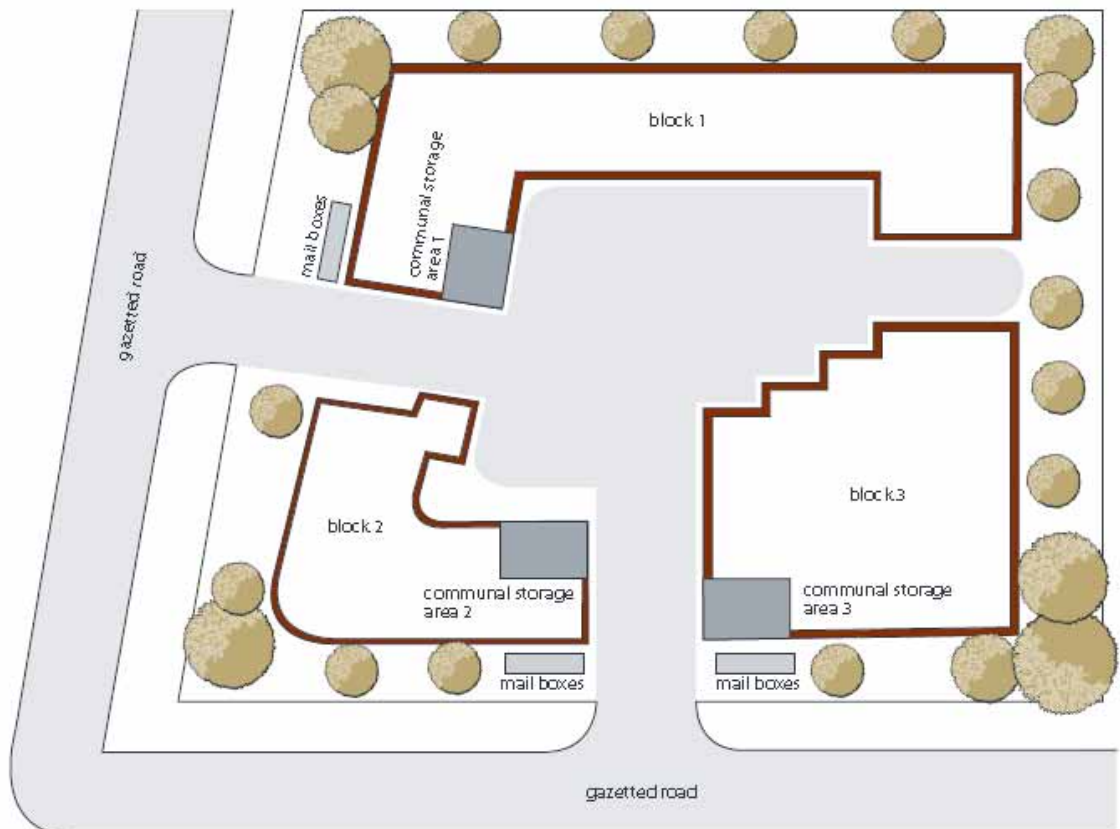
Figure 6: Example of Communal Storage Area for Bulk Bins suitable for Low Rise Developments
