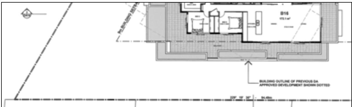
Figure 2 - Setback encroachment levels 5 and 6 in tower “B” adjacent to southern boundary
