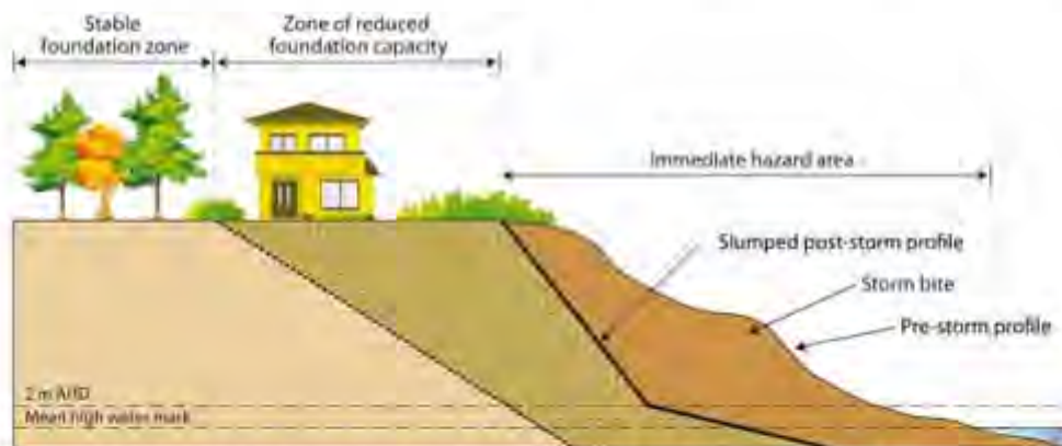
Figure 3.2. Idealised schematic of a dune profile depicting the immediate hazard area and associated zone of reduced foundation capacity (after Nielsen et al 1992).
