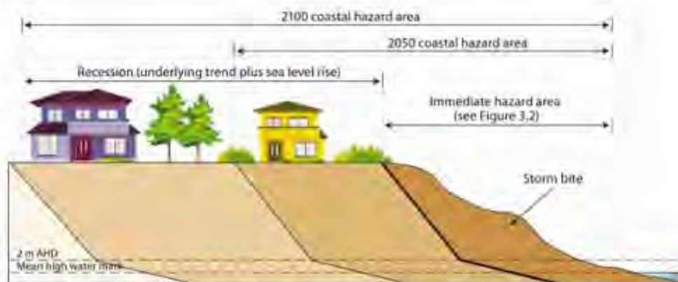
Figure 3.3. Idealised schematic of a dune profile depicting the high hazard area, 2050 coastal hazard area and 2100 coastal hazard area.
