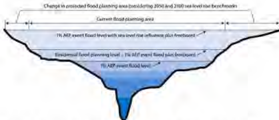
Figure 4.1. Flood levels, flood planning areas and the influence of the sea level rise benchmarks (cross-section view).
