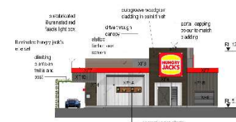
NORTH ELEVATION - DRIVE THRU
