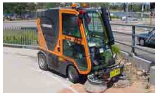
Figure Bicycle path sweeping machine Source: NSW Bicycle Guidelines, 2005
