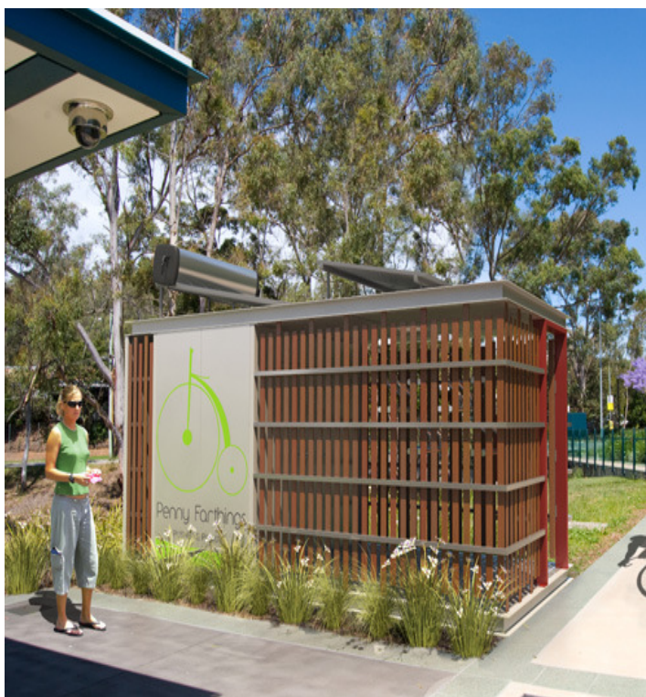
Figure 6.1.7c: The Green Pod is the size of one car park space and comes in two configurations; 1 Shower, 1 Change Room, 10 Bicycles, 10 Lockers or 2 Showers, 2 Change Rooms, 28 Lockers, 0 bicycles
