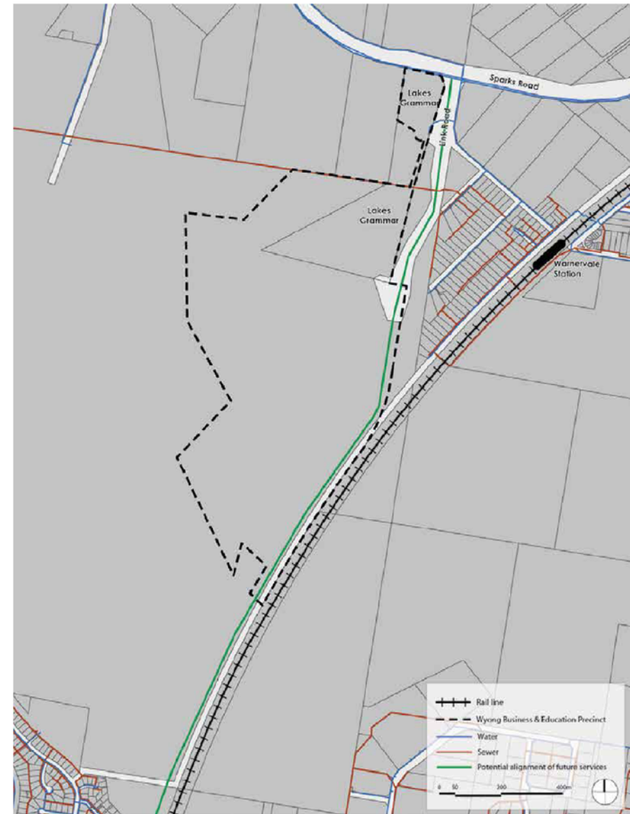
Figure 14 - Infrastructure features of the proposed site.
