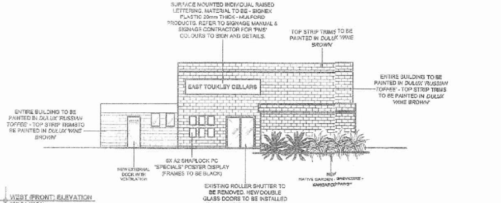
WEST (FRONT) ELEVATION SCALE 1:100@A1
