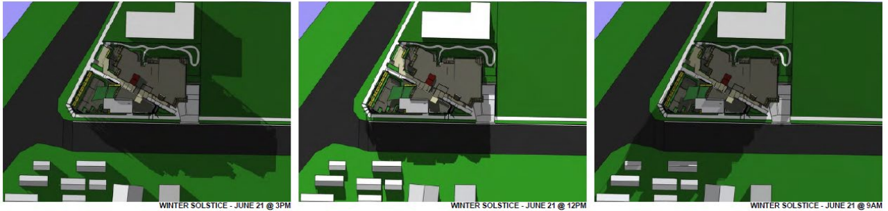
Figure 14: Shadow diagrams for the proposal midwinter at intervals of 9am, midday and 3pm.
