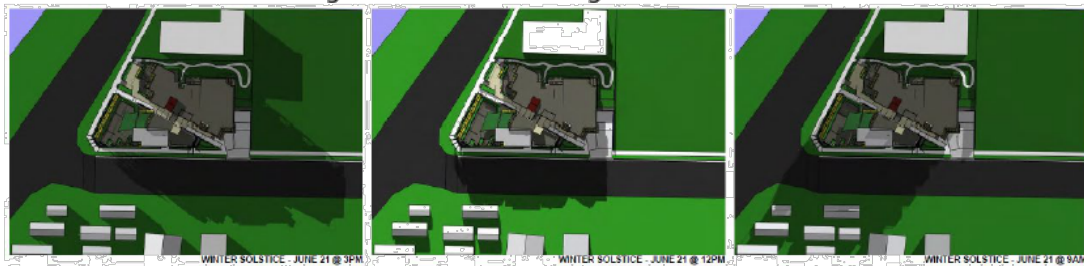
Above: Shadow diagrams for the proposal midwinter at intervals of 9am, midday and 3pm.
