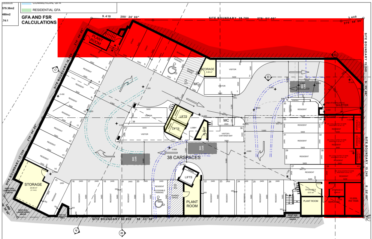
Figure 11 – Areas on non-compliance 6m deep soil setback
