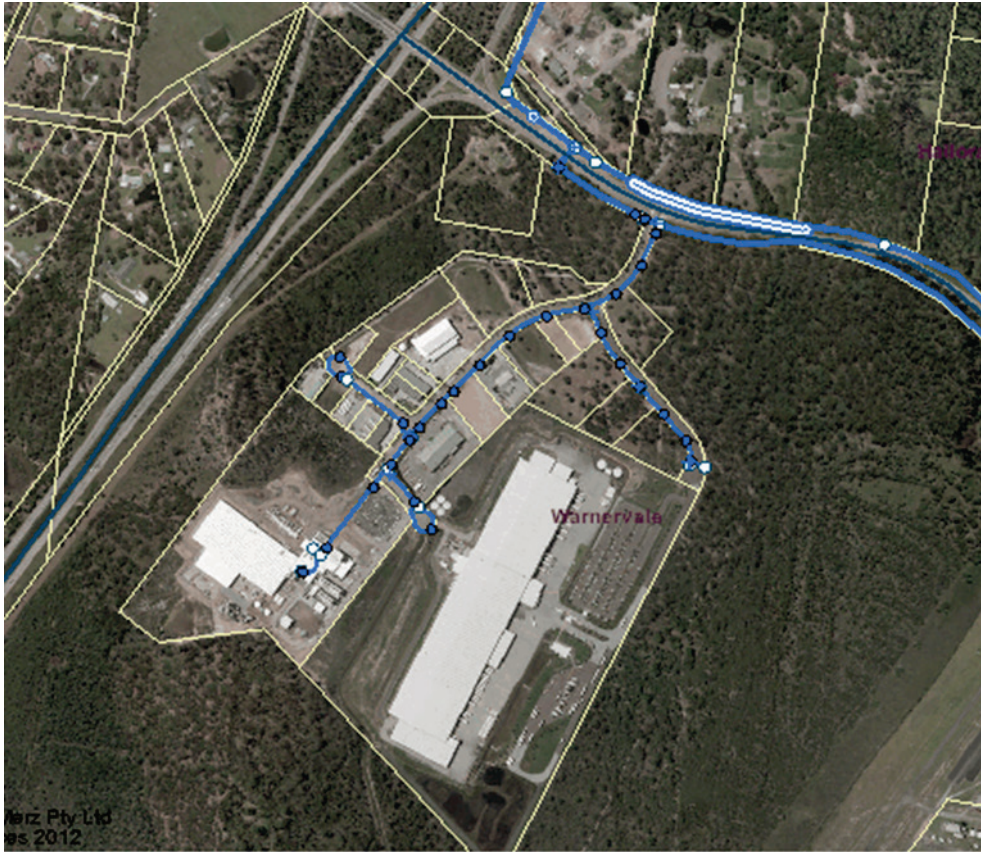
Figure 1 Water mains in the locality
