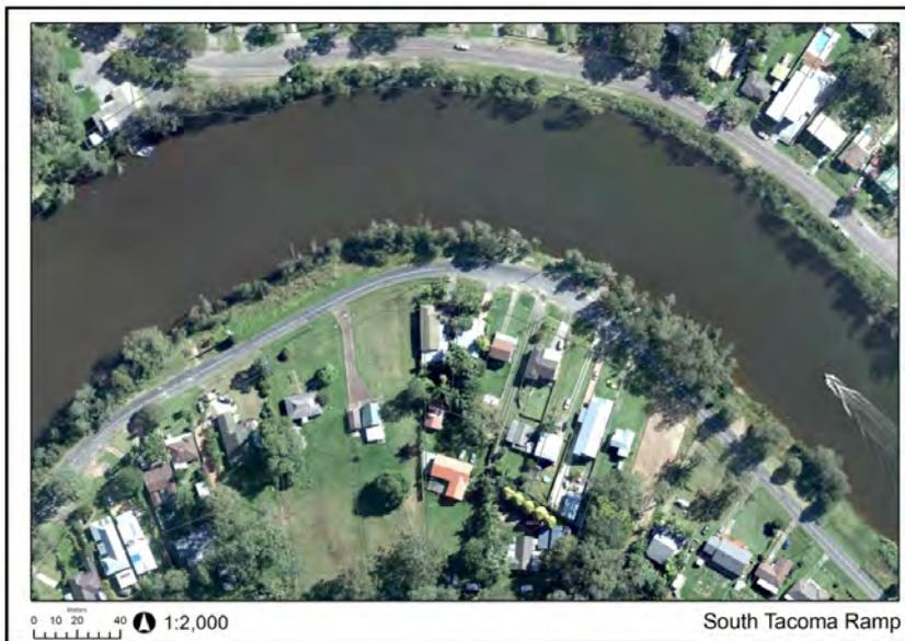
Local ramp on Wyong River with no parking in a dangerous location requiring access on a road travelling land. Requires relocation.
