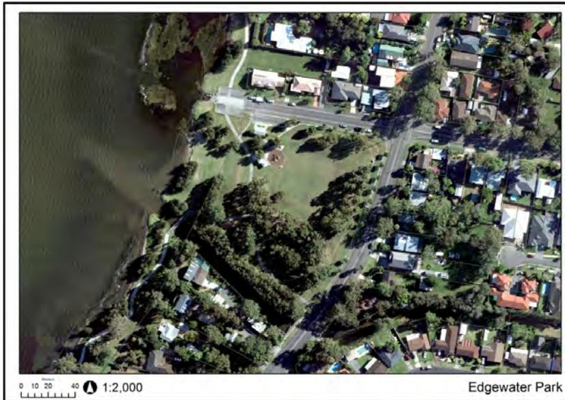
A local public ramp with no dedicated trailer parking on Budgewoi Lake. The ramp is subject to wrack accumulation due to the inlet design. Adjacent to a well-developed park.
