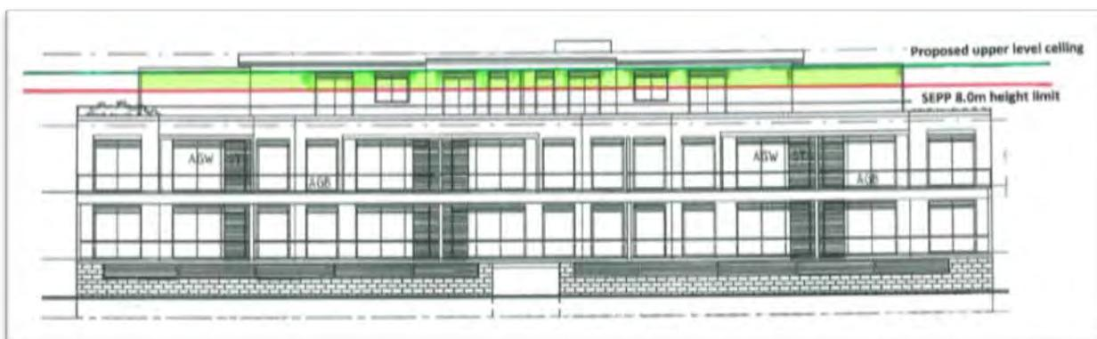
**Figure 4:** image of building block with green shading representing part of building above limit SEPP height
