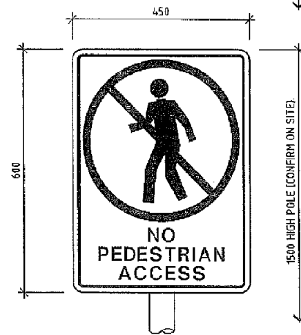
S7 CAR PARK SIGNAGE SG010 NON-ILLUMINATED ALUMINIUM REFLECTIVE SIGN ON GALVANISED STEEL POLE TYPICAL.
